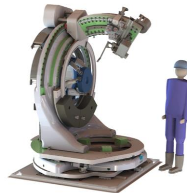
CEA: diffractometer to study nanostructures growth
