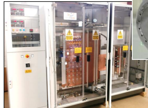
CRYRING Kicker magnet and pulser
