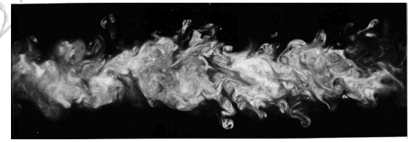
Turbulent wake of a cylinder
