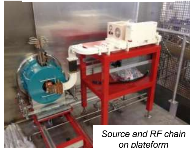
Accelerating column and ion source with coils
