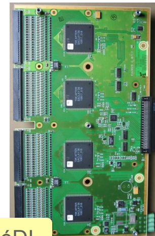
Front-End card with 4 AGET* chips
