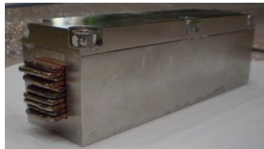
Reaction mold for Nb 3 sn cable thickness variation studies
