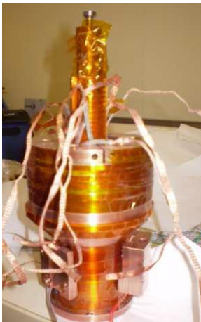
Solenoidal pancakes of superconducting tapes for quench propagation studies
