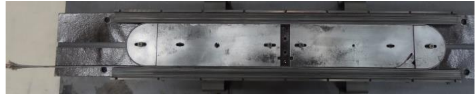
Reaction molds for dimensional changes studies and stress control in Nb 3 Sn coils
