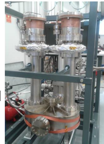
2 prototype couplers on the test bench at INDRA (Madrid). Photo : CIEMAT
