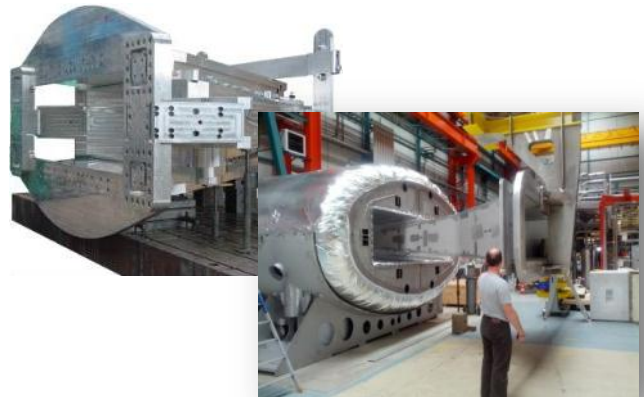
R3B magnet mechanical design : cold mass & vacuum vessel
