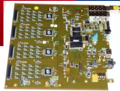
512-channel front-end unit (x 50)
