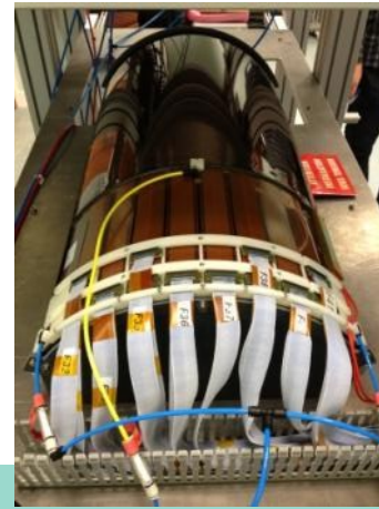
Barrel detectors 20k channels, 6 layers, 3\ \text{m}^2 detection area Self-sustained curved tiles
