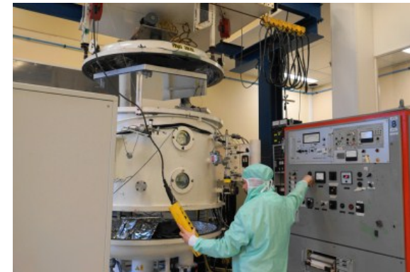
Mirror being removed from vacuum chamber after coating at KERDRY
