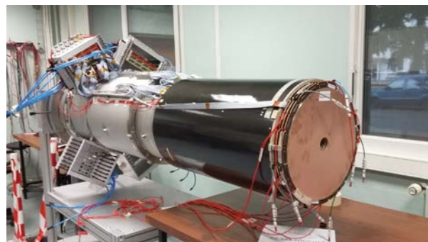
Figure 1 : Cylindrical Micromegas tracker for CLAS12 under construction at IRFU.
