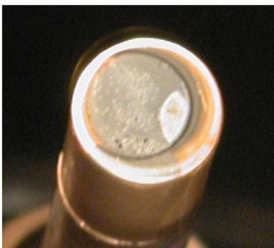
Fig. 9: Photograph of a  $\text{Cs}_2\text{Te}$  photo cathode.
