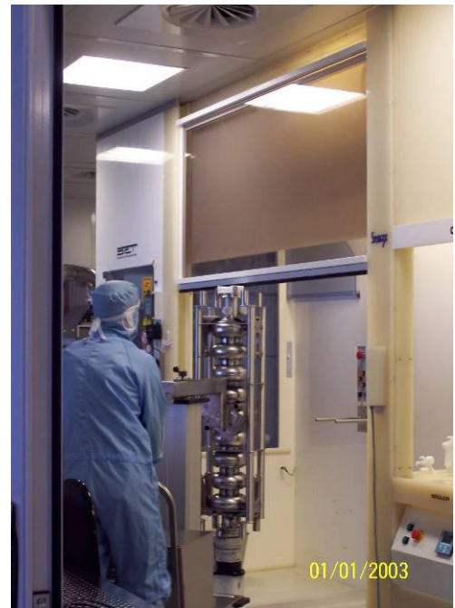
Cavity after EP being transferred into the clean room
