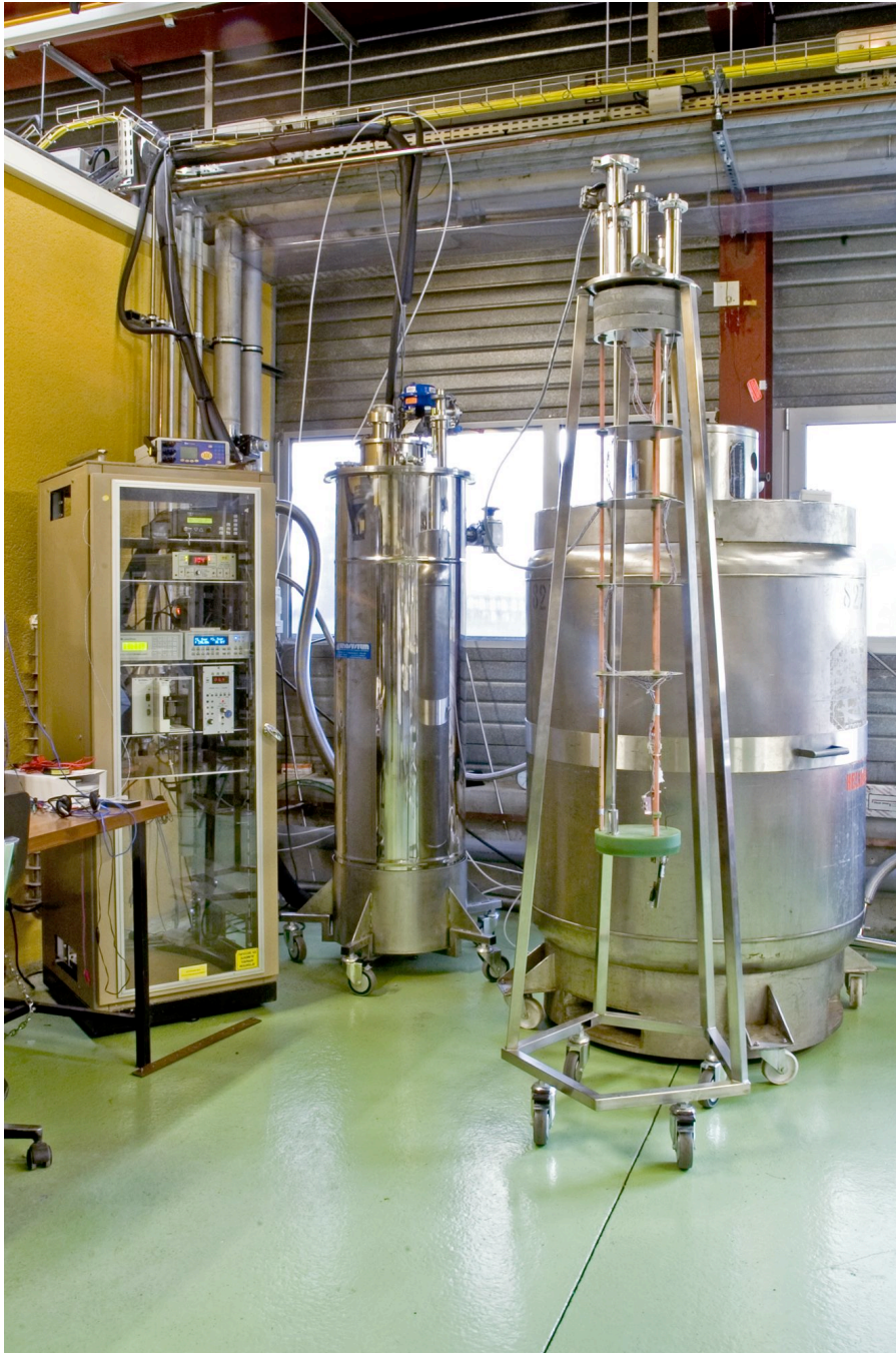
Figure 3. The NED Facility at CEA Saclay. The Automation and data acquisition system is located on the left. The cryostat it self is located in the middle of the Photo and on the right side of the picture one can see the 500 litres Dewar and the insert where the Lambda plate can be seen.
