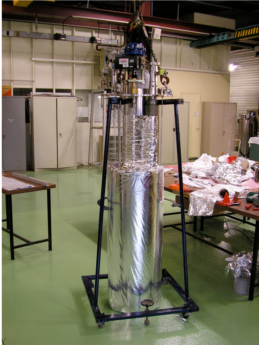
Figure. 2. Preparation of the Cryostat for Vacuum test and leak detection. The picture shows the inner vessel with super-insulation to be removed for the tests.
