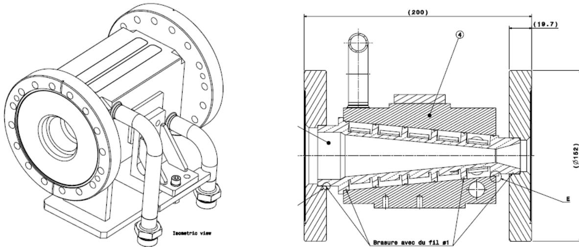
**Figure 6** – Isometric view and cross-section of the absorber [6].
