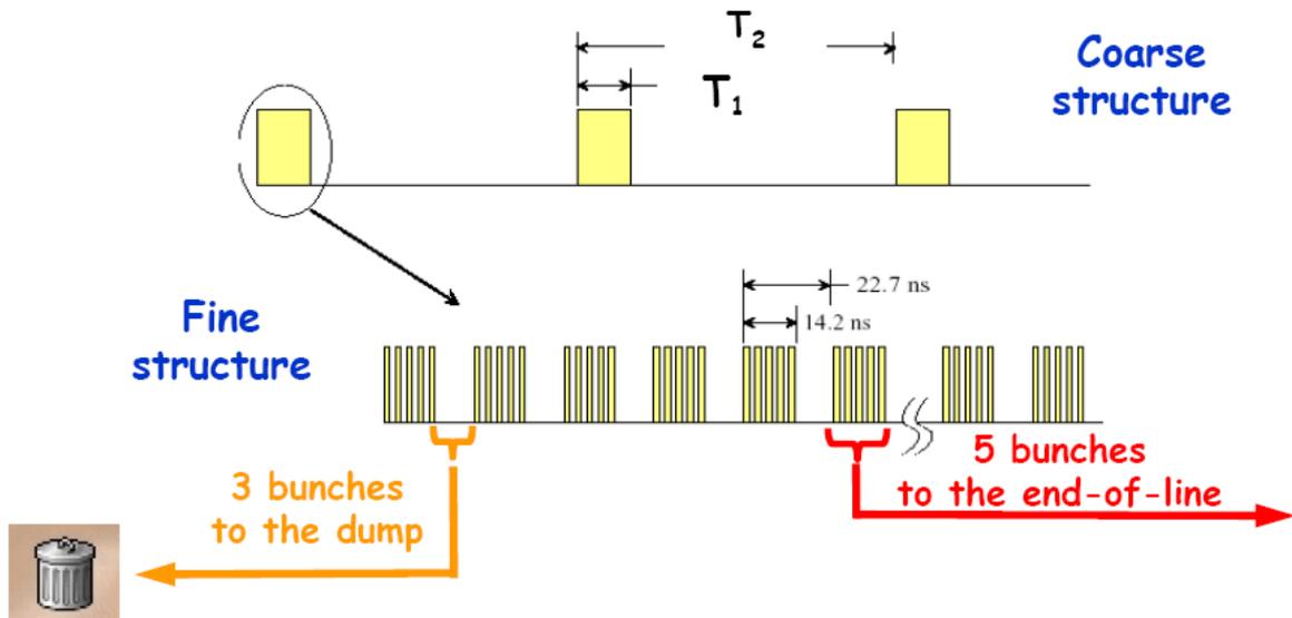
Figure 3 – Time structure of the 3 MeV  $\text{H}^-$  beam.
