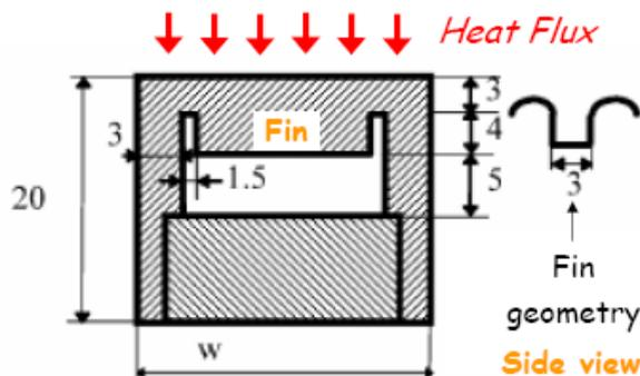
**Figure 7** – Schematic cross-section of a cooling channel (dimensions are in [mm]).
