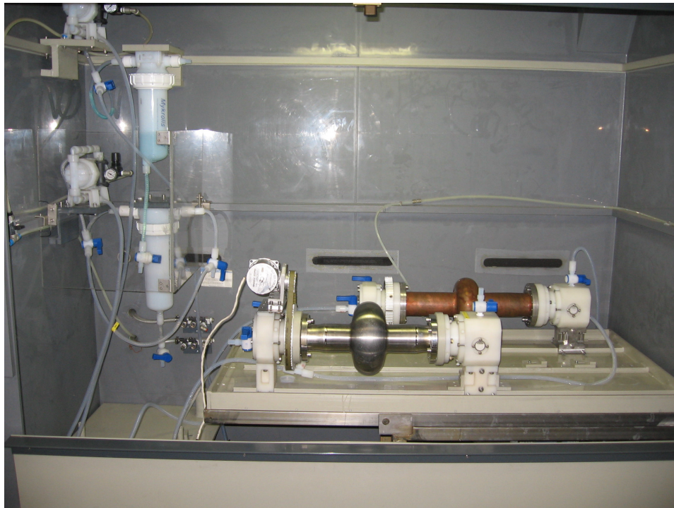
Fig. 5: The rotating cavity EP system built for the treatment of both Niobium and Copper.
