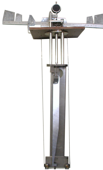
Fig. 8: The mechanical arrangement of the test bench with the tuner lever and link to be tested.
