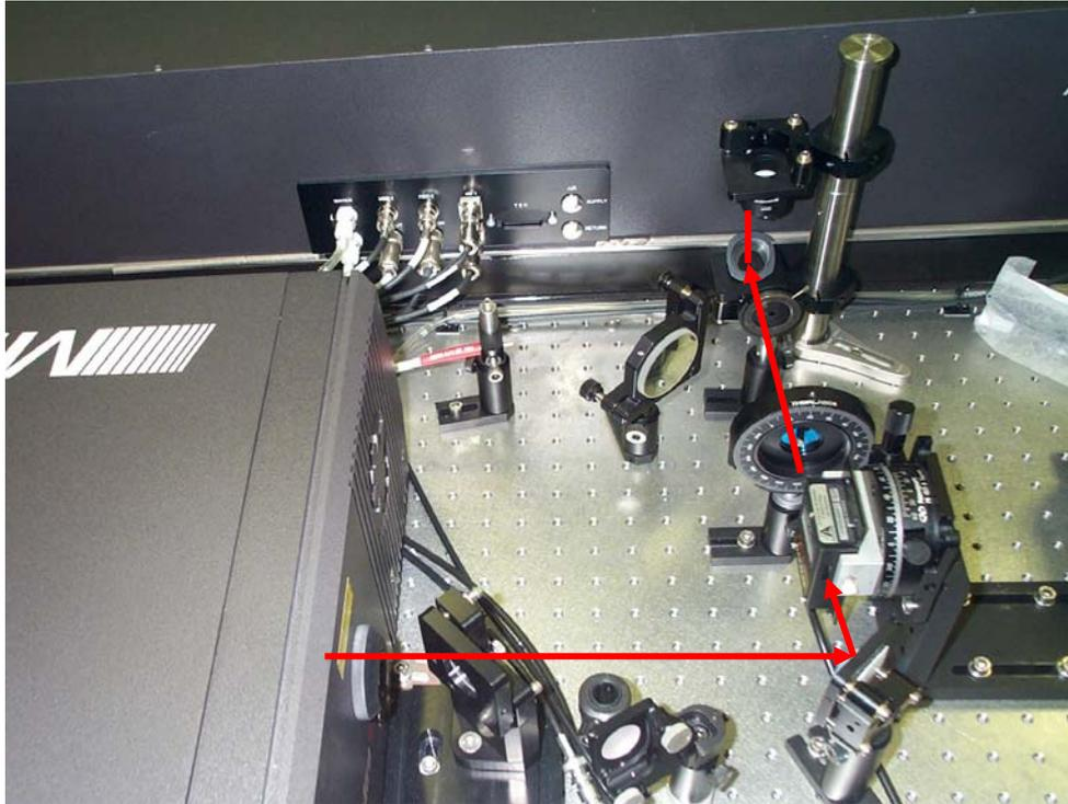
Figure 1. Dazzler set-up: the oscillator output is sent to the acousto-optic filter and a half wavelength wave-plate. After, a periscope is used to inject the beam in the amplifier.
