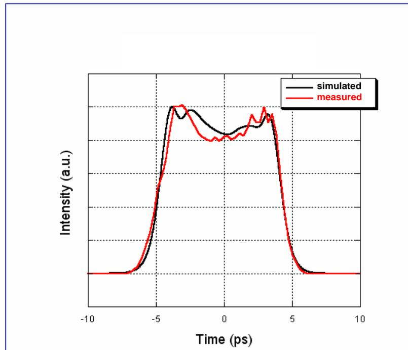
Numerical simulations indicate that to further reduce the rise time it is important to increase the spectral width of the UV pulse. This requires a dedicated work to replace the non-linear crystal with thinner ones.
