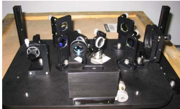
Figure 3 Picture of the third harmonic generator.
