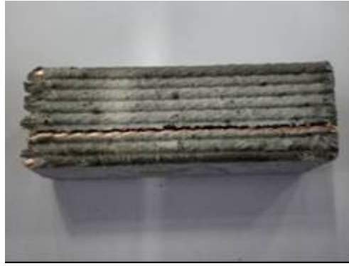
Fig.7: Stack of insulated cables reacted with a pre-compression, after outing of the reaction mould and relaxation of the cable stack
