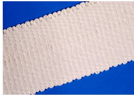
Fig.2: Innovative insulation tape with ceramic precursor.
