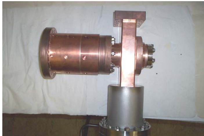
Figure 4: AlphaX RF gun which will be installed in the NEPAL test beamline.
