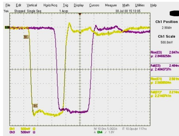
Figure 24: Chopper input and output waveforms Yellow: chopper input, red: chopper output, 100 V/div, 10 ns/div
