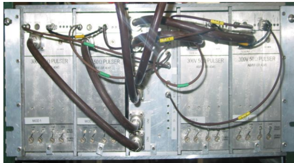
Figure 15: CERN driver \pm 250 V prototype.
