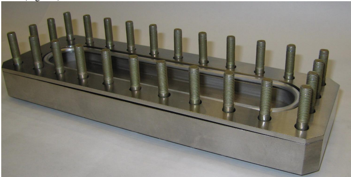
Figure 8 Flange test set-up for vacuum tests with "racetrack" Helicoflex gaskets
