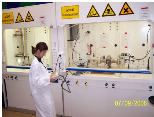
Figure 8a : The EP facility bench with set-up with remote control for pneumatic valves.
