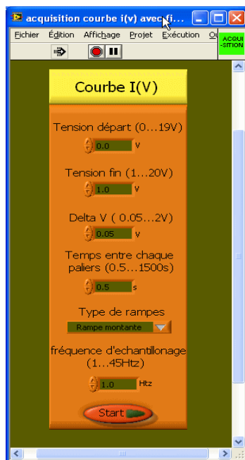
Figure 15a : Parameters chosen for I(V) curves plotting: voltage boundaries, frequency, scan rate, possible reverse scan.
