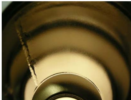
Figure 28: Internal surface of 1C21 cavity after 130 \mu\text{m} removal with EP at 5 volts.
