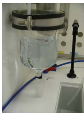
Figure 11a : Scrubber filled with BTB.
