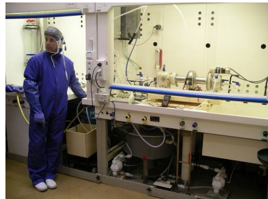
Figure 8b : Saclay EP set-up during a cavity treatment.
