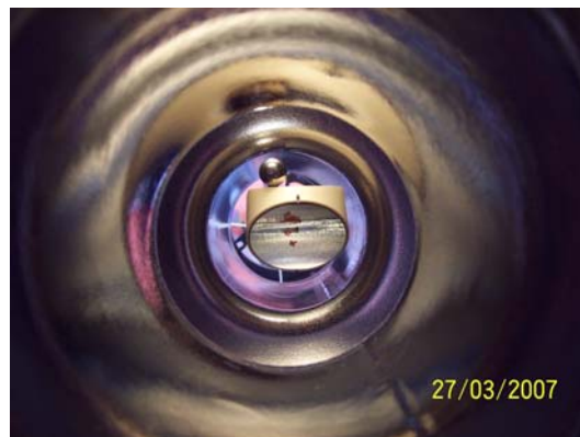
Figure 25: Copper deposition on the surface of the cavity. Origin from the copper cathode.
