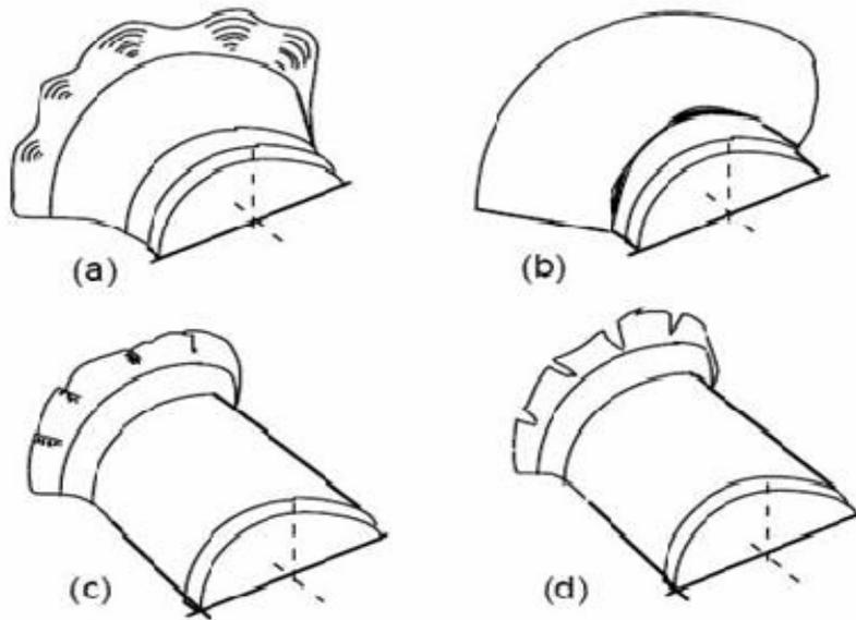
Figure 9: Typical failures in spinning:
