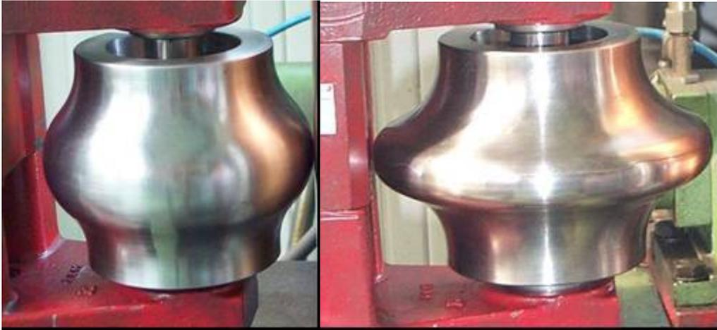
Figure 6: Rollers for spinning Niobium cavities: left for the start of the spinning, right for final forming small curvatures at the iris or transition region of cavity to beam pipe.
