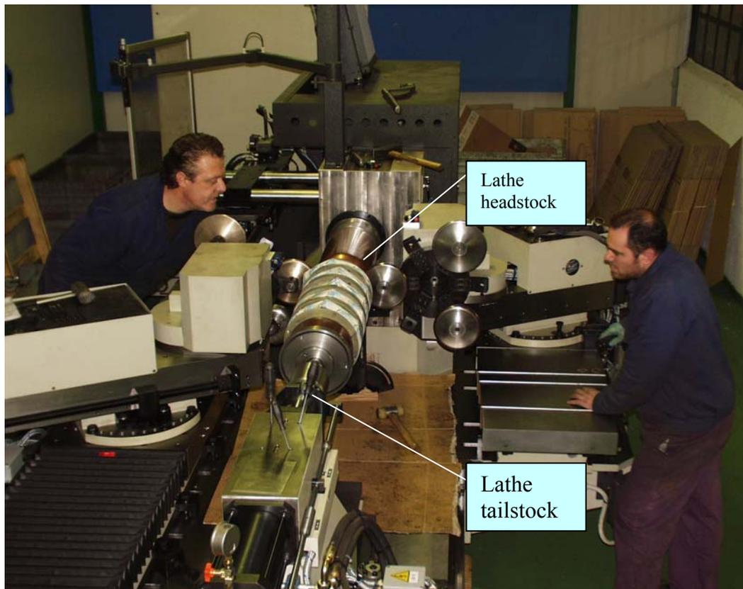
Figure 5: The spinning lathe in the laboratory.
