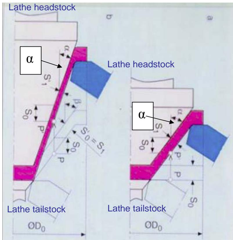
Figure 4: Dependence of the material thickness “S” on the spinning angle  $\alpha$
