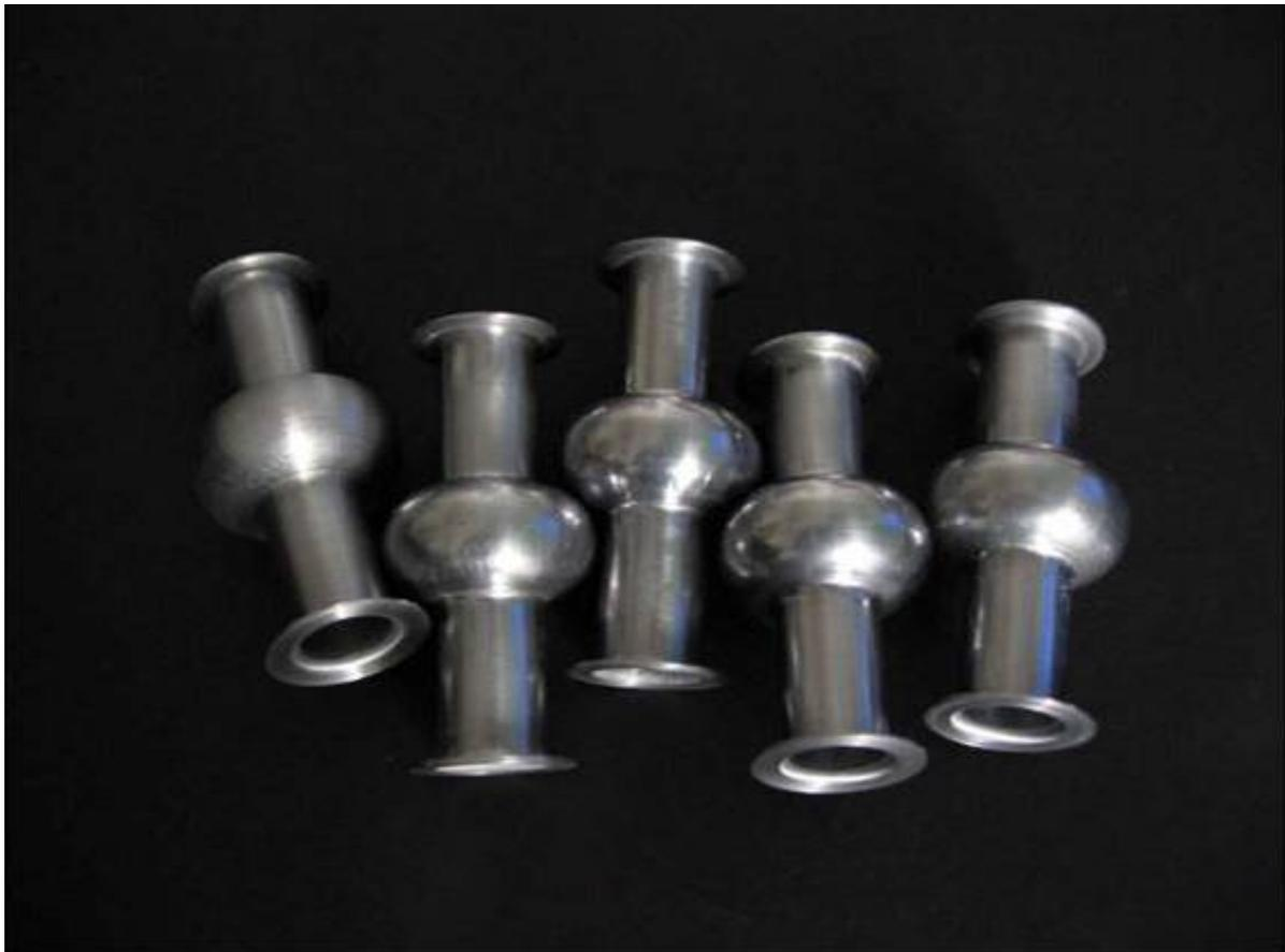
Figure 2: Examples of single cell cavities fabricated by spinning. Please note the integrated flange construction which results in a totally seamless cavity fabrication process.
