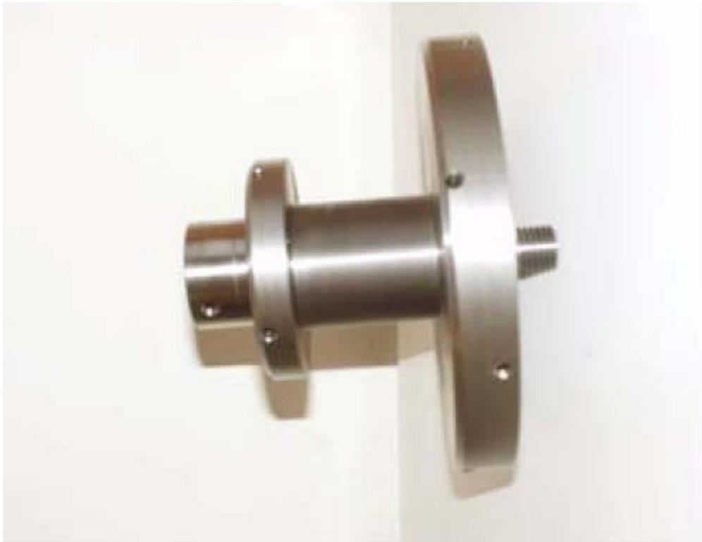
Figure 7: Tool to regulate the operational distance between headstock and tailstock
