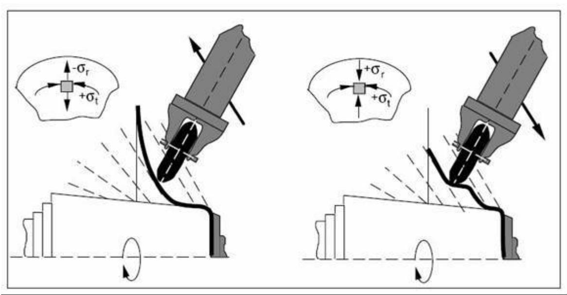
Figure 8: Forming process during moving towards or away from the blank support
