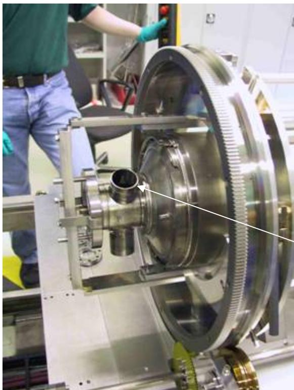
Figure 14: Welding fixture for the exchange of the older Niobium flange system with the new NbTi design.
