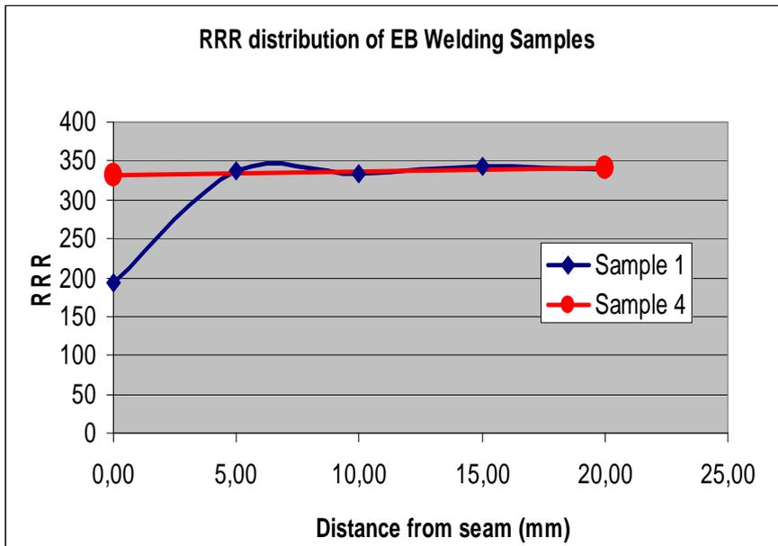
Figure 7: RRR in the welding seam area with (sample 4) and without (sample 1) of Nb evaporation in the EB chamber (DESY+Julich)
