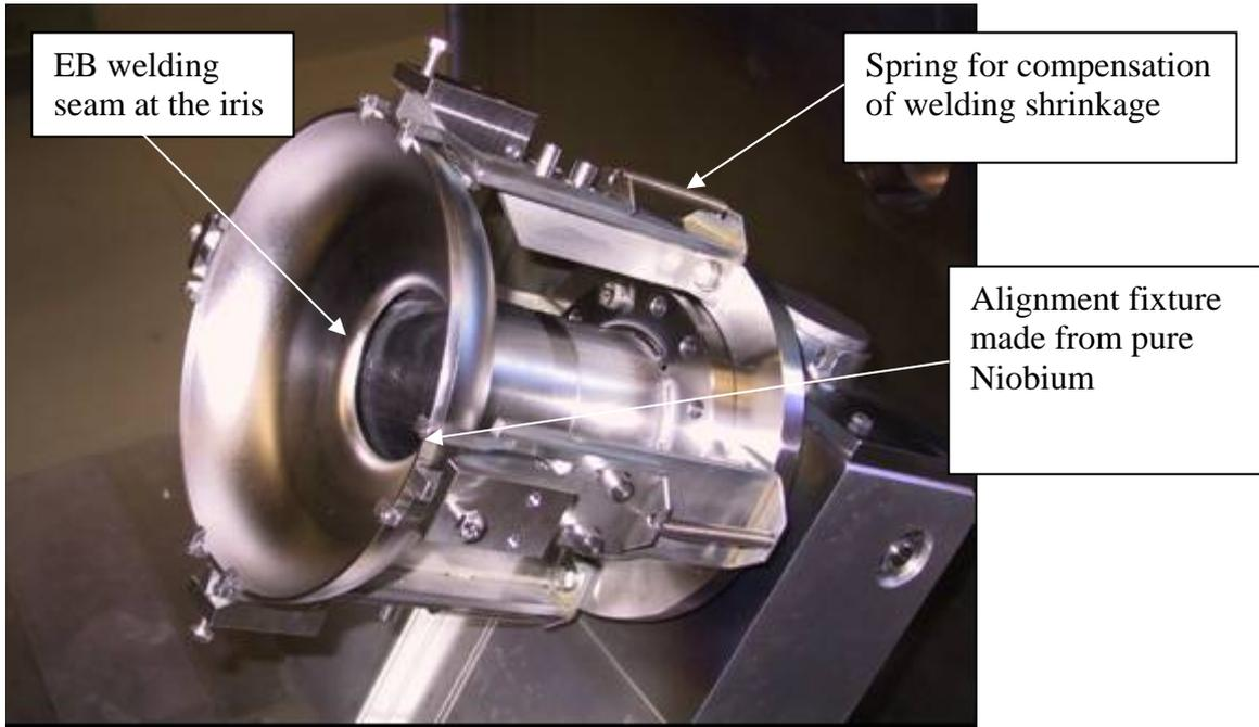
Figure 10: Welding tool for the cell to beam pipe connection
