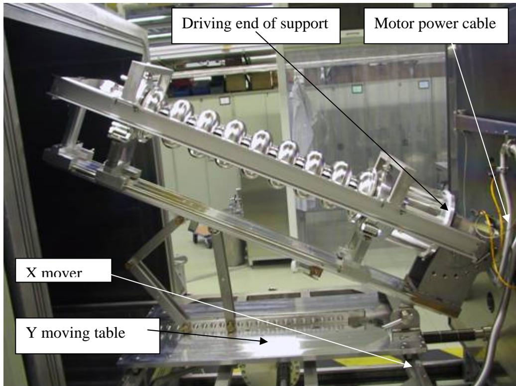
Figure 12: Complete support for 9-cell cavity welding at the DESY EB facility
