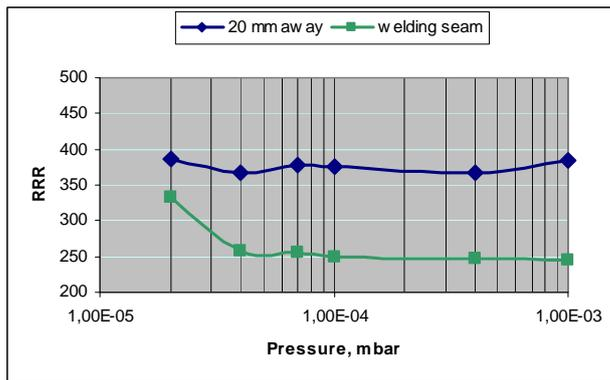
Fig.:4 RRR in the welding seam and 20 mm away versus pressure in the chamber during EB welding (company I)
