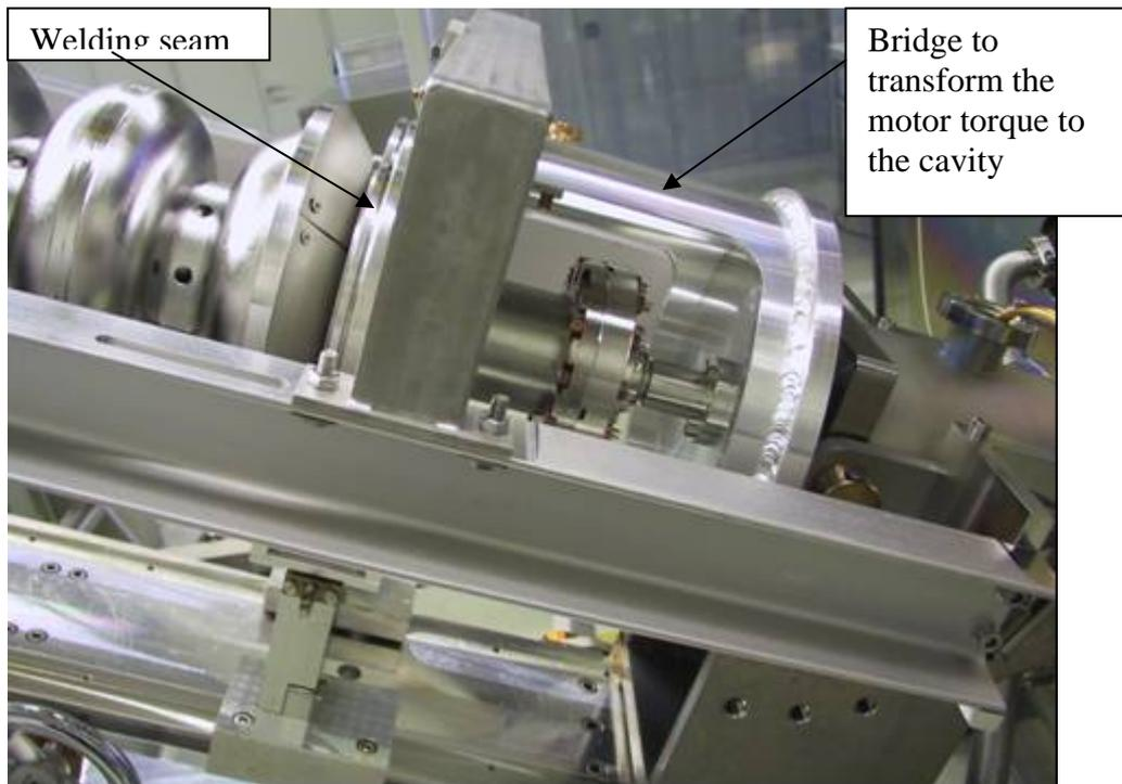
Figure 13: Details of the driving end of the welding fixture for multicell cavities. In this picture the EB weld at the outer end of the conical head disc is performed.
