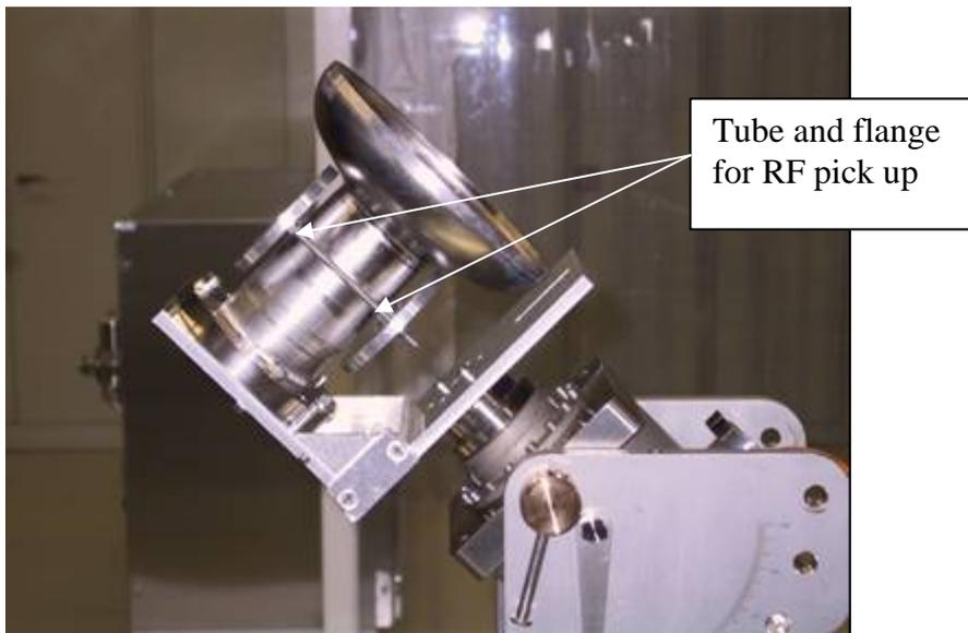
Figure 11: Welding tool for the flange welding at the pick up signal line
