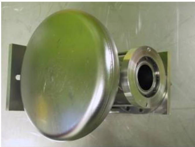
Figure 9: Picture of a one cell RF gun cavity (phase velocity of 0,6)
