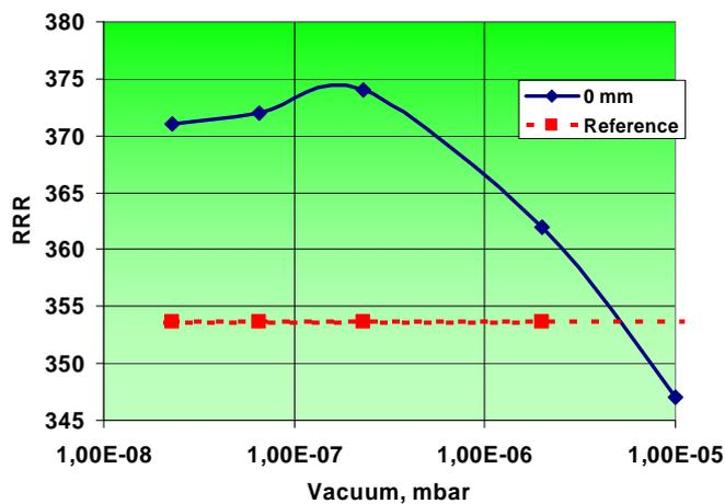
Figure 6: RRR sample measurements at the DESY welder at improved static vacuum
