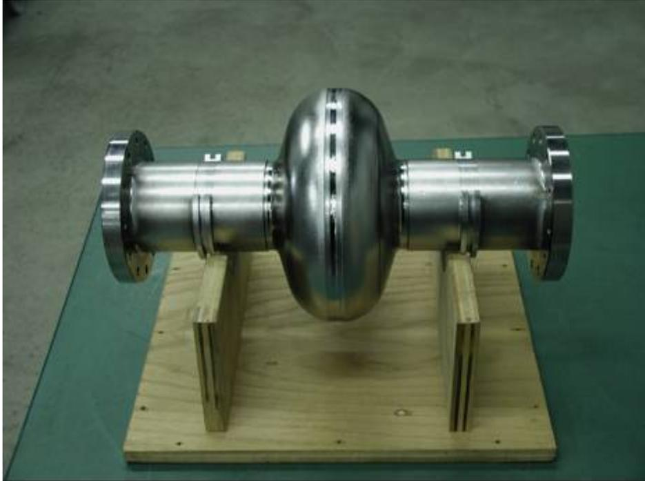
Figure 8: Standard 1-cell cavity design at 1.3 GHz (TTF shape). The flanges are of the same design as the TTF 9-cell cavity. The two sets of rings at the beam pipe serve as a fixture for the mechanical support of the cavity during preparation and cold test.
