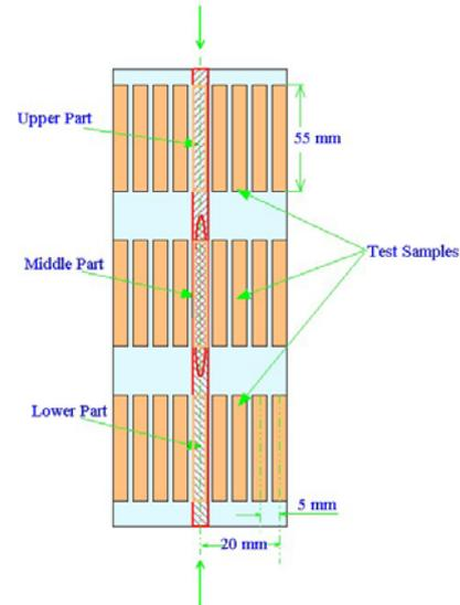
Fig 3: Scheme of the RRR samples cut off
