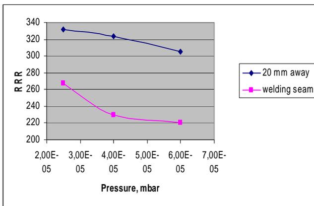
Fig.: 5 RRR in the welding seam and 20 mm away versus pressure in the chamber during EB welding (company II)
