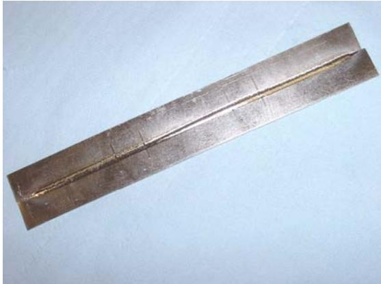
Fig 2: Example of Nb welding strip
