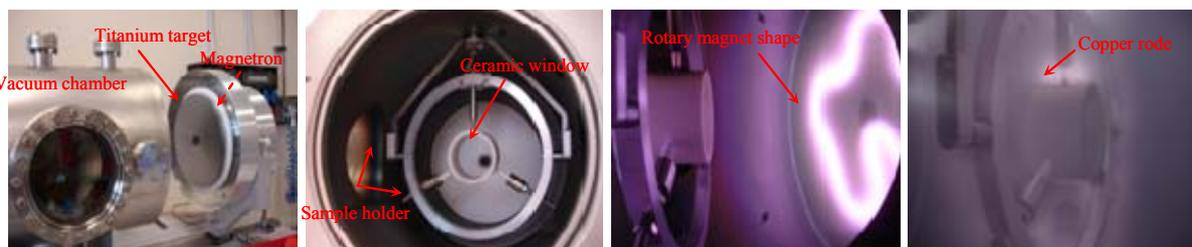
Figure 6: Components of sputtering machine
