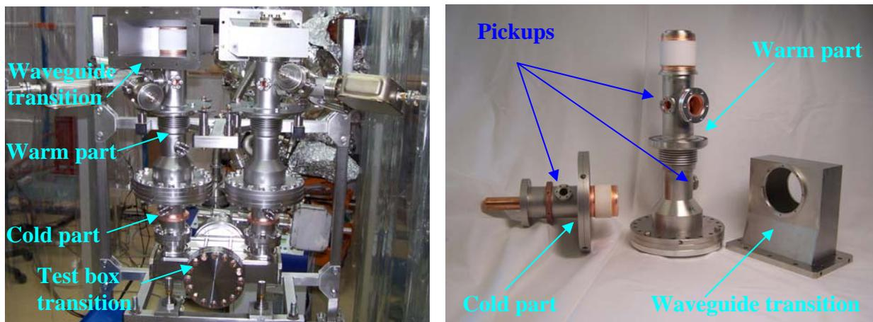
Fig. 2: TTF-V coupler. The photo at the right shows the main coupler parts. The photo at the left shows an assembly of a pair of TTF-V couplers using a test box transition.
