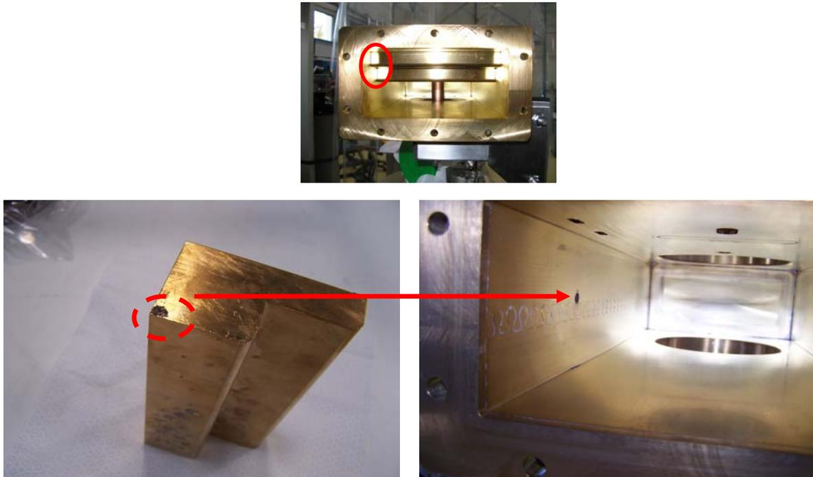
Fig. 9: Some arcs taking place in the waveguide transition of the TW60 during processing.
