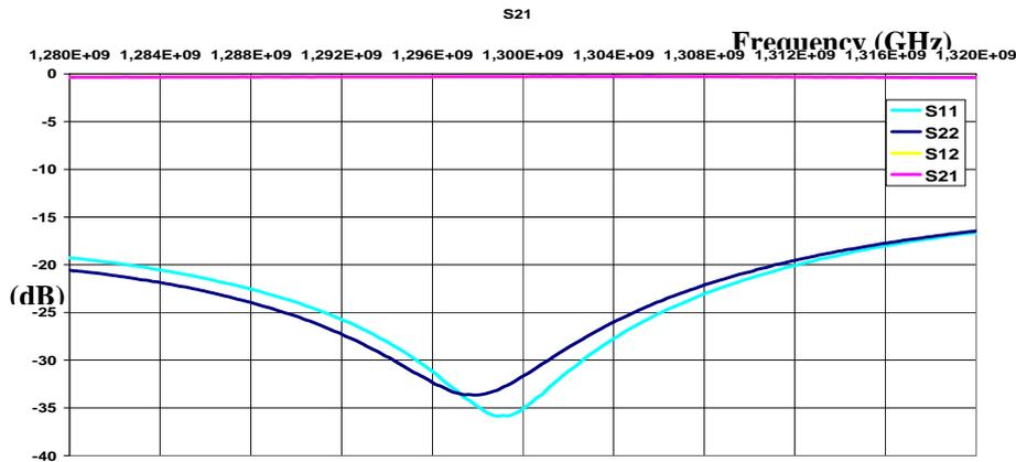
Fig. 3: Low level RF measurements on a TTF-V coupler pair with the new test box transition.
