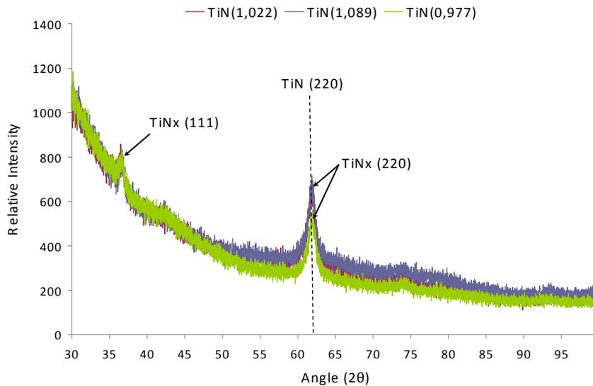
Figure 7: XRD plot for different TiNx deposits- comparison to stoichiometric film
