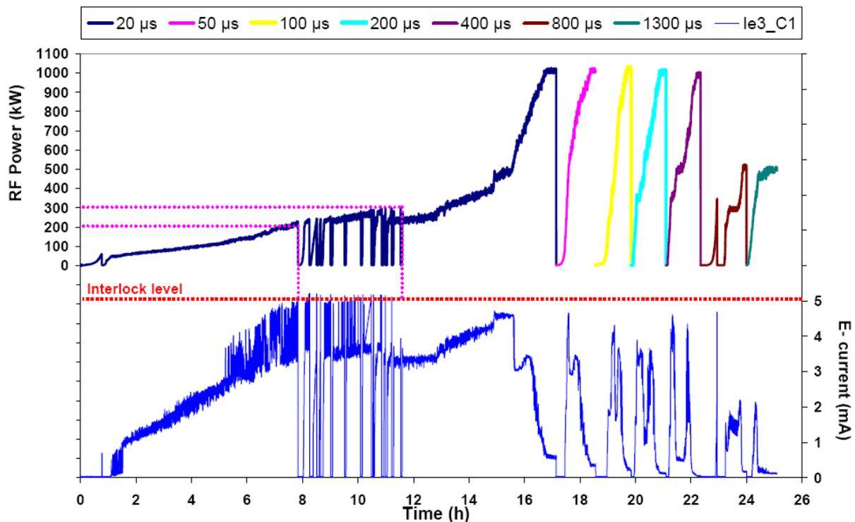
Fig. 10: Power variation during RF conditioning and interlock events. Ie3\_C1 is the  $e^-$  current detected with the pickup of the upstream coupler cold part.
