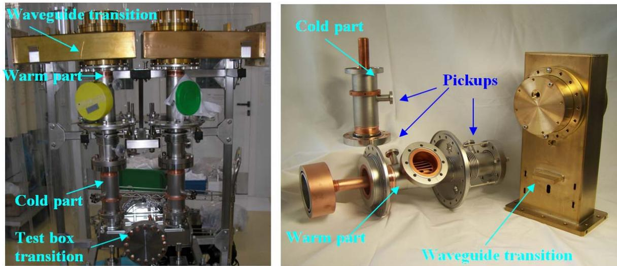
Fig. 1: TW60 coupler. The photo at the right shows the main coupler parts. The photo at the left shows an assembly of a pair of TW60 couplers using a test box transition.
