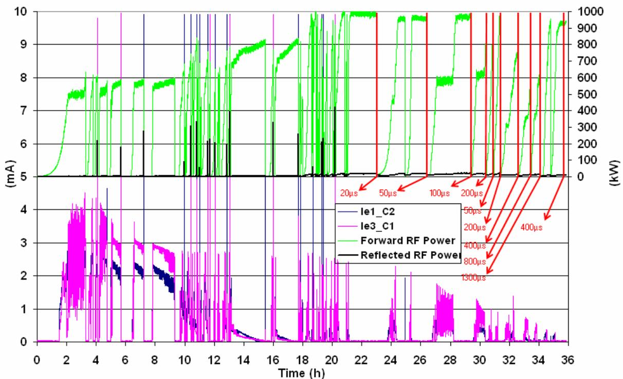
Fig. 8: Power variation during the RF conditioning of a TW60 coupler pair in June 2008. We can see the strong correlation between the  $e^-$  currents jumps with the reflected RF power. We only illustrated the behavior of the  $e^-$  current pickup of the cold part in the upstream coupler (Ie3\_C1) and the  $e^-$  current pickup near the warm window in the downstream coupler (Ie1\_C2), which were at the origin of the majority of the interlocks.
