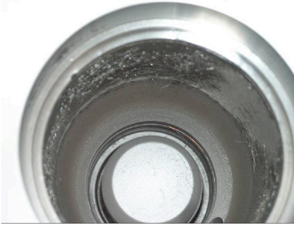
**Fig.6** – Peeling on the anode in the cathodic region
