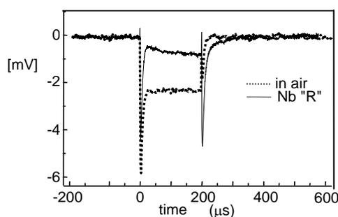
Figure 8 : A magnetic pulse signal detected by the Hall probe in air (dot line) and in presence of a Niobium sheet (straight line).
