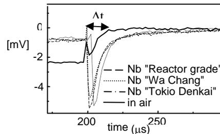
Figure 9: A magnetic pulse signal detected by the Hall probe in air and in presence of three different Niobium test samples.
