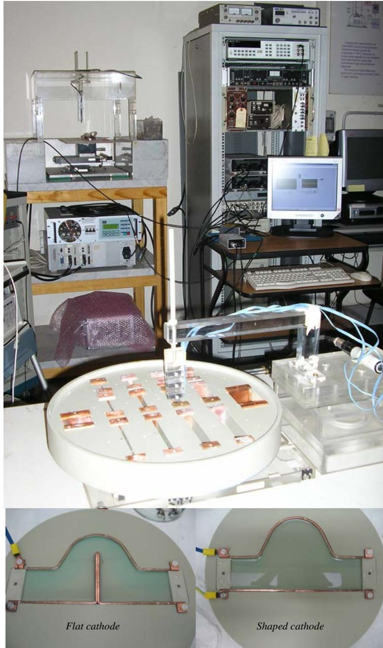
Figure 1 : The electrolytic cells monitored: above are the rectangular cells, below a cavity section with flat and shaped cathode, respectively.
