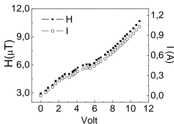
Figure 2 : H-V and I-V polarization curve.
