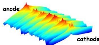
Figure 4: the current distribution for the rectangular cells at the potential of 4 V.
