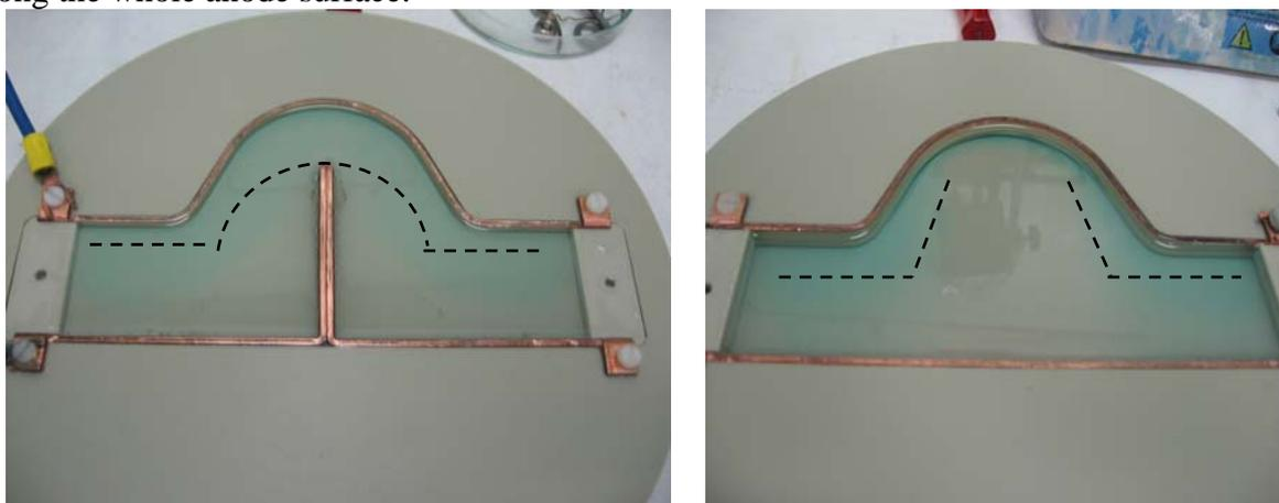
Figure 7: The electrolytic cells analysed: a cavity like electrode with flat and shaped cathode, respectively. The dot lines follow the viscous layer due to uniform electropolishing process.
