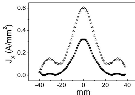
Figure 6: Comparison of the corresponding current density for lines scan extracted from the magnetic maps of fig 4. (squares) flat cathode and (triangles) shaped cathode.
