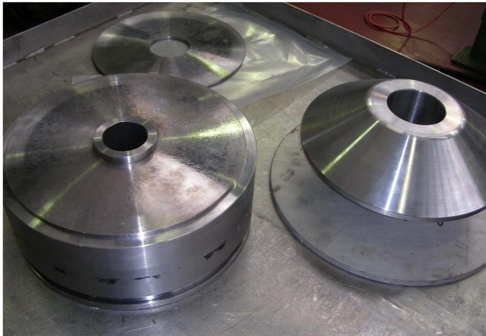
Figure 27: tool for NbTi end dish deep drawing
