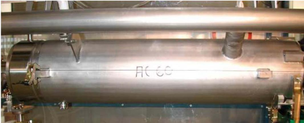
Figure 1: the TTF cavity ready to be installed in the cavity string.
