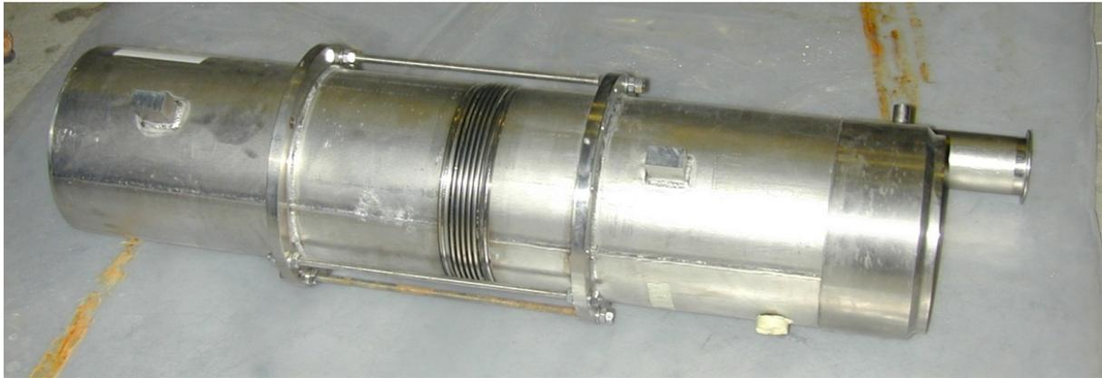
Figure 5: the modified He tank. The safety rods, installed between the welded rings, are temporarily placed to save the bellow from unwanted deformations.
