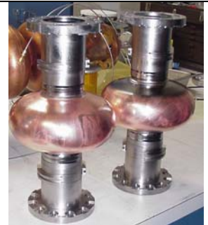
Fig. 18: Two cavities in preparation for tests
