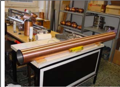
Fig. 16: Bimetallic tube clad by niobium and Cu0.15%Zr alloy
