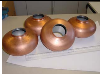
Fig. 17: Single cell cavities produced from Nb Cu0.15%Zr tube
