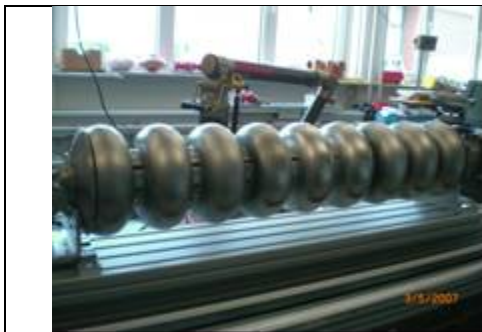
Fig. 14: Hydroformed 9-cell TESLA cavity Z145
