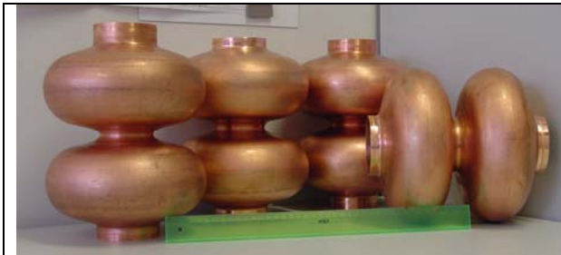
Fig. 19: Double cell NbCu clad cavities produced at DESY by hydroforming from KEK tubes
