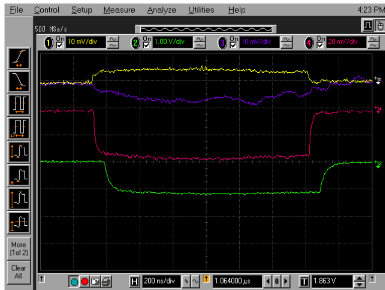
Figure 7: Signals from BPR (H, V, S) and Faraday Cup Horizontal (Yellow), Vertical (Magenta), Sum (Red), FCU (green) Pulse length 1300 ns.
