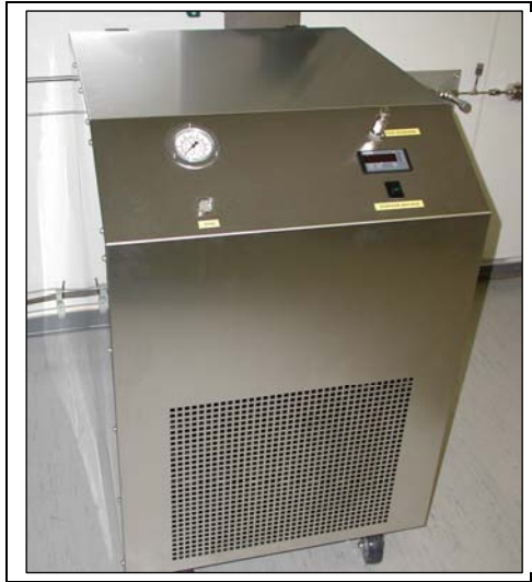
Figure 10: CO 2 - cooler/purifier unit (left) and horizontal motion unit with the spraying cane assembled on the linear drive (right)
