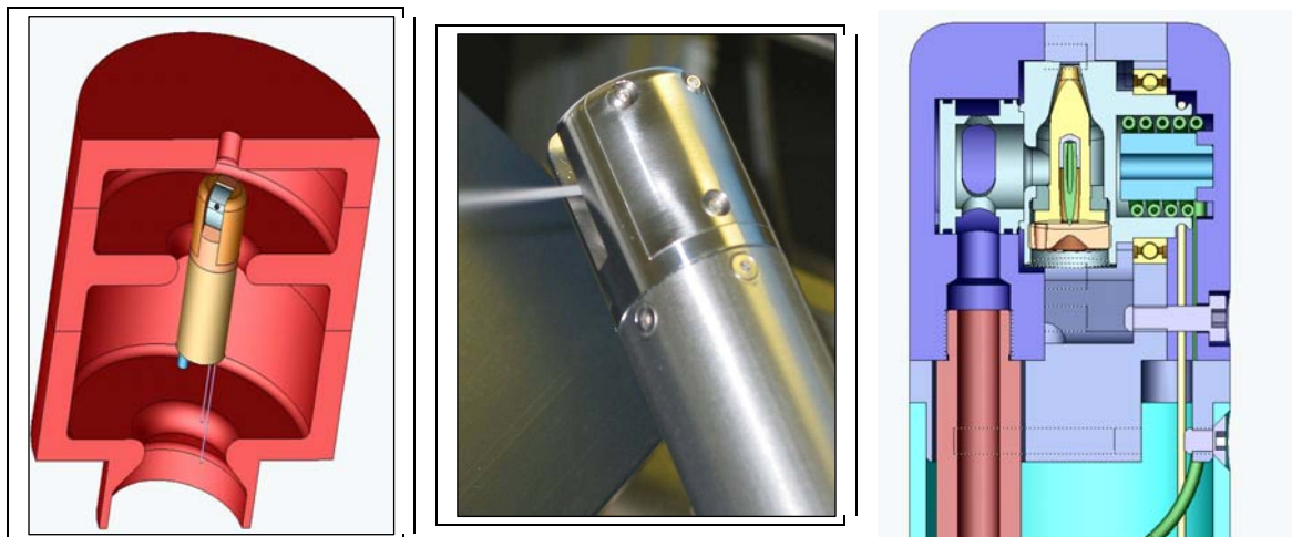
Figure 16: 3D-model of gun cavity with rotatable nozzle (left); rotatable nozzle (middle); cross-sectional view of the nozzle
