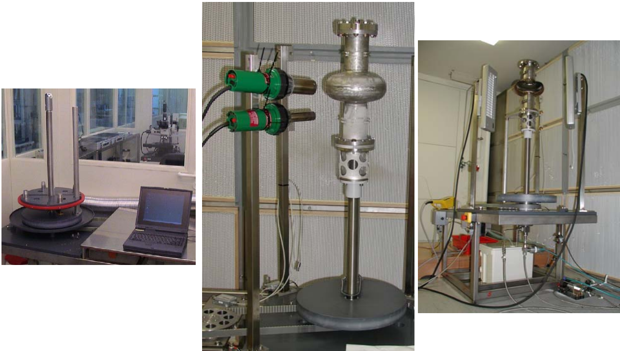
Figure 6: Vertical set-up for pre-tests on single-cell cavities at Fraunhofer IPA (left) and DESY (middle + right)
