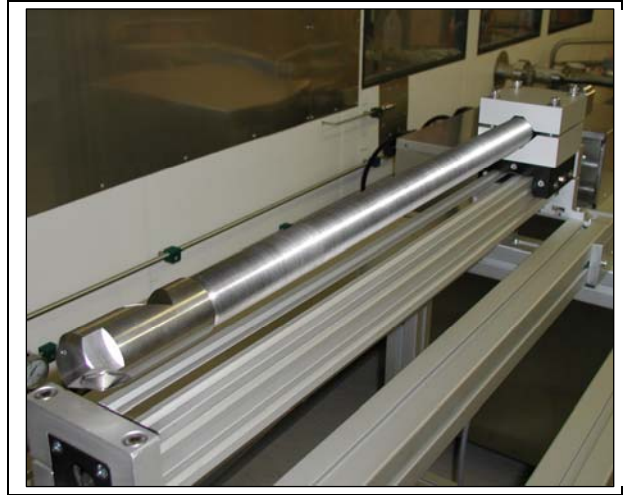
Figure 10: CO 2 - cooler/purifier unit (left) and horizontal motion unit with the spraying cane assembled on the linear drive (right)
