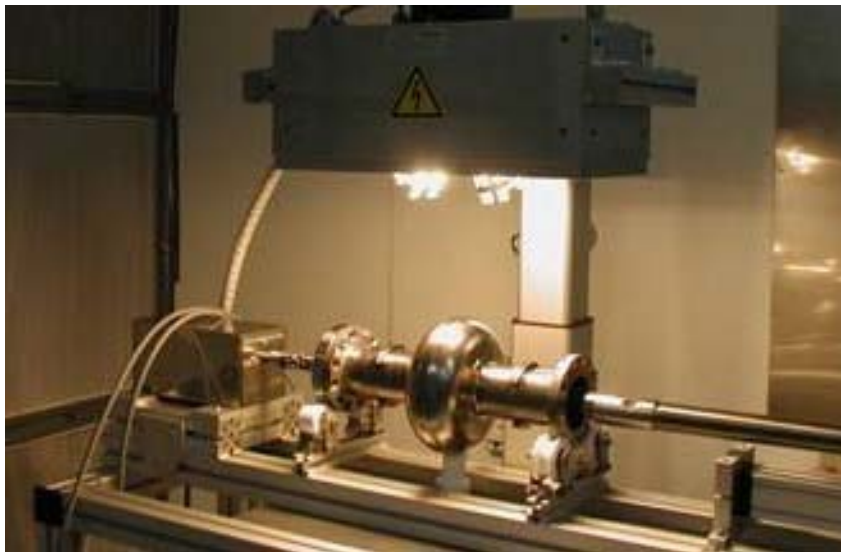
Figure 11: Dry-ice cleaning system with IR heater in upper rest position and horizontal nozzle system. The exhaust system (not visible) acts from the bottom close to the open cavity flange.
