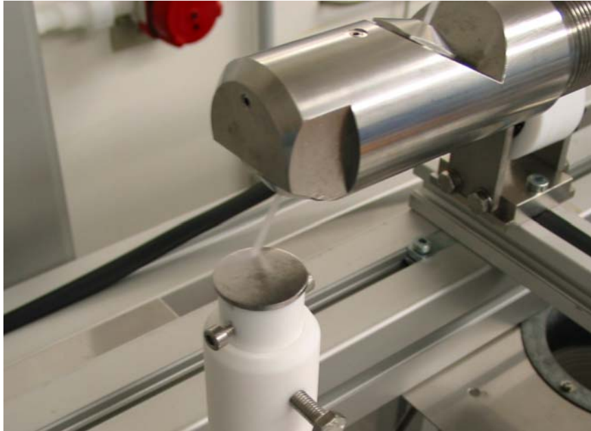
Figure 14: Cleaning of a Nb sample for the investigation of field emission properties within the frame work of WP 6.3
