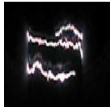
*Fig.4. General view of the modified UHV linear-arc system (left) and a picture of a stable arc discharge (right), as observed on the cylindrical cathode at the base pressure of  $4 \times 10^{-10}$  mTr, arc current of 40 A, during the discharge lasting 1 minute.*
