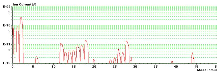
Fig.3. Mass-spectrum of residual gases, recorded at the final pressure  $p = 1.5 \cdot 10^{-10}$  mbar, as achieved after 180-hour pumping and 30-hour backing at  $T_b = 150^\circ\text{C}$ .
