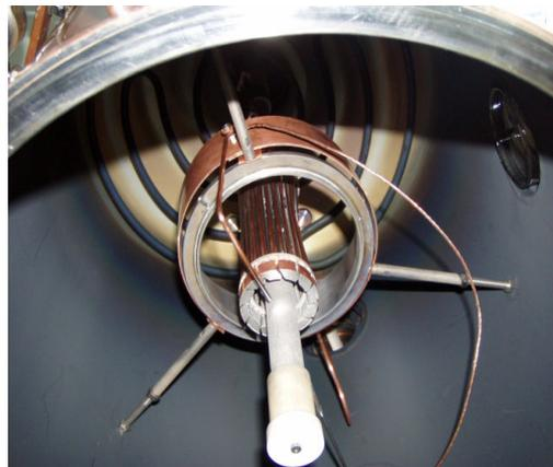
*Fig.15. Picture of the cylindrical magnetic filter and an additional anode after the exploitation tests.*
