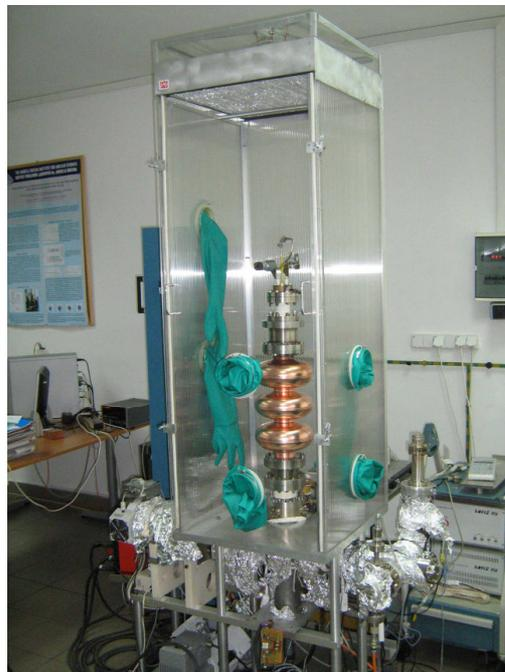
*Fig. 22. UHV linear arc facility before commissioning for the first coating of a test triple-cell.*
