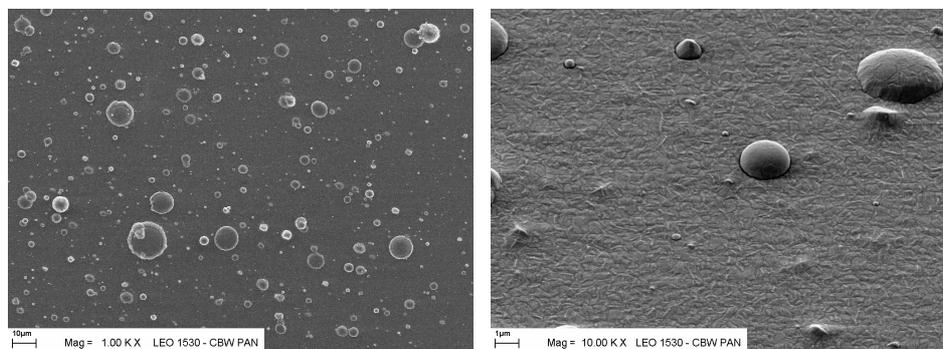
*Fig.11. SEM pictures showing the population of the deposited micro-droplets (left), as well as the structure of the Nb-layer and shapes of micro-droplets (right, larger magnification).*
