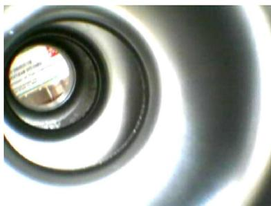
*Fig.23. End-on picture of the model triple-cell cavity coated with Nb layer.*
