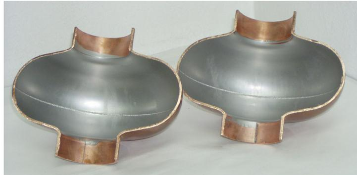
*Fig.9. Two parts of the coated single-cell, which show the Nb layer on the inner surfaces.*
