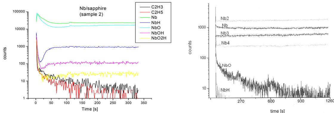
Fig.17. SIMS profiles of the Nb films deposited without any micro-droplet filter, which were recorded with the use of the oxygen ions (left) and argon ions (right).
