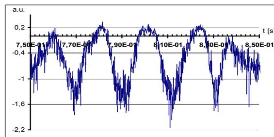
*Fig.8. Waveforms of the discharge current, as recorded during laboratory tests of the UHV linear-arc facility.*
