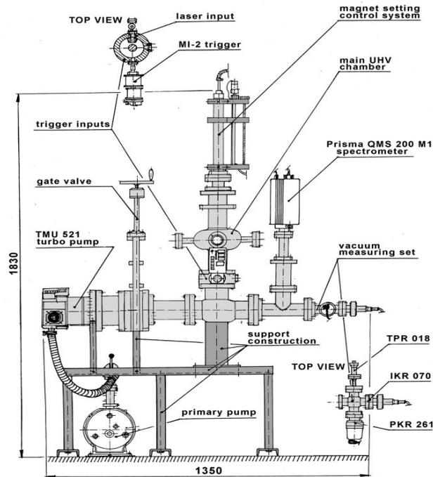
Fig.2. Scheme of the modified UHV stand equipped with the linear-cathode arc system.
