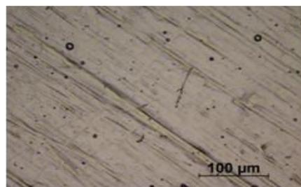
Fig.26. Surface of the Nb-layer deposited upon a polycrystalline copper sample, as observed after HPWR at 120 bars.
