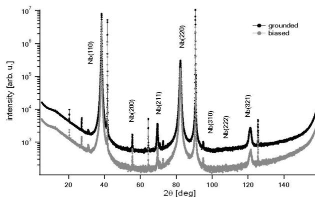
*Fig. 20. X-ray diffraction patterns from Nb layers deposited upon the biased- and grounded-samples.*
