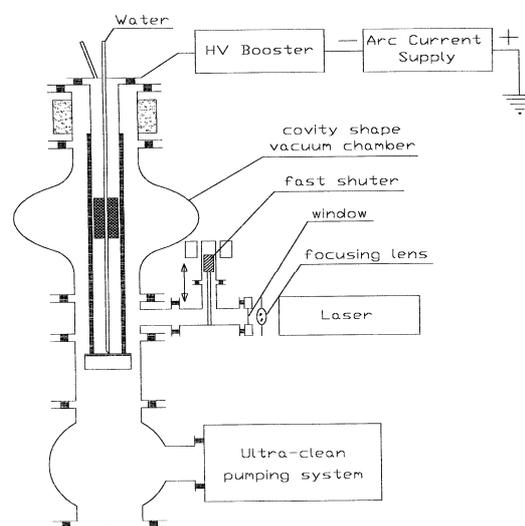
*Fig.1. Scheme of an UHV facility designed for the linear-arc cathode coating.*
