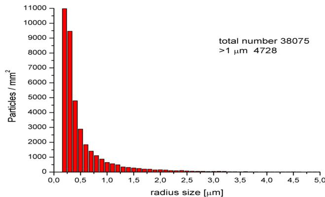
*Fig.12. Histograms of the micro-droplet population, as measured upon the sapphire sample coated within the UHV linear-arc facility.*
