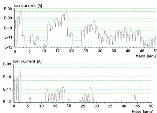
*Fig.5. Typical RGA mass-spectra recorded within the linear-arc facility, as recorded before and after 24-hour baking at 150 °C.*
