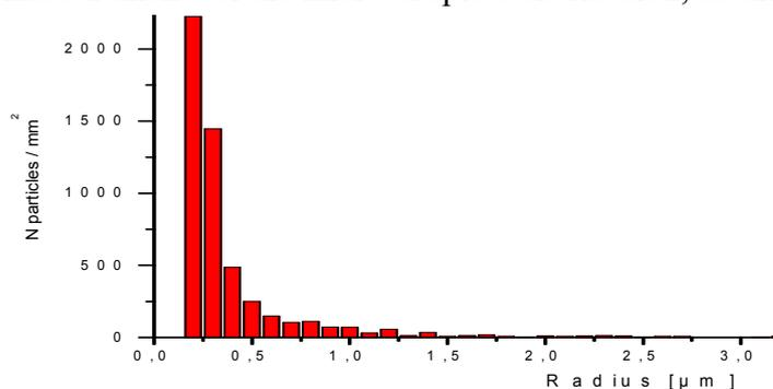
Fig.18. Population of micro-droplets upon the filtered Nb-layer.
