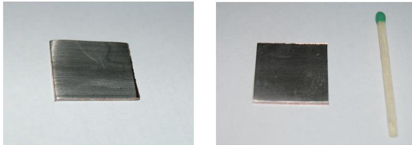
Fig.25. Nb-coated Cu-sample (left) and the same sample after the HPWR at 100 bars (right).
