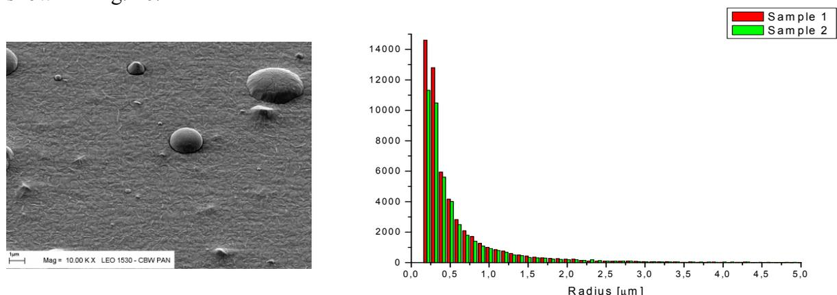
Fig.16. SEM picture of an unfiltered sample and numbers of the deposited micro-droplets.
