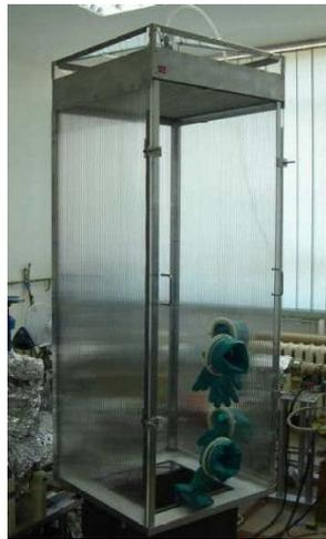
*Fig.19. Removable laminar flow chamber equipped with operation al gloves.*
