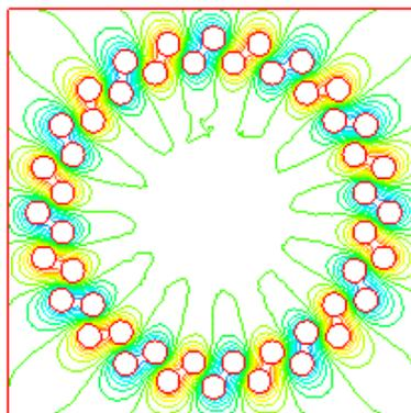
*Fig.13. Distribution of magnetic field lines in the horizontal cross-section of the cylindrical magnetic filter, which consisted of 24 pairs of current-carrying tubes.*
