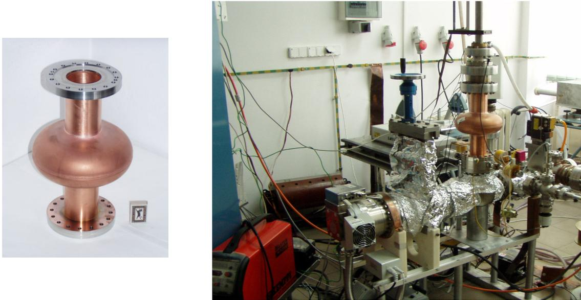
*Fig.7. Single copper-cavity with end flanges (left) and the modified UHV linear-arc system during laboratory tests of the single-cavity coating (right).*
