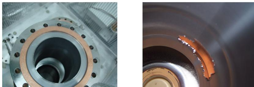
*Fig. 21. End-on picture of the second cavity from CEA-Saclay, as taken after its coating (left), and a picture taken after the cleaning process at CEA-Saclay, which shows some destruction of the Nb-layer by high-pressure water rinsing.*
