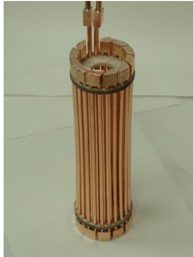
*Fig.14. General view of the cylindrical magnetic filter with connections for magnetizing current and cooling water flows.*
