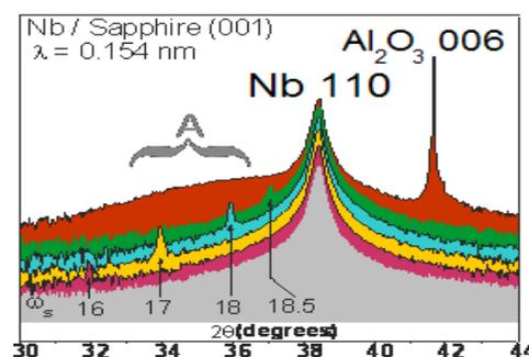
Fig.27. Nb-110 reflection measured for the Nb/sapphire film. The upper pattern represents results of the symmetric  $\omega$ - $2\theta$  scan, where two components of peak profile are clearly seen. The other patterns were measured in a detector scan at the fixed incidence angle  $\omega_s$ .
