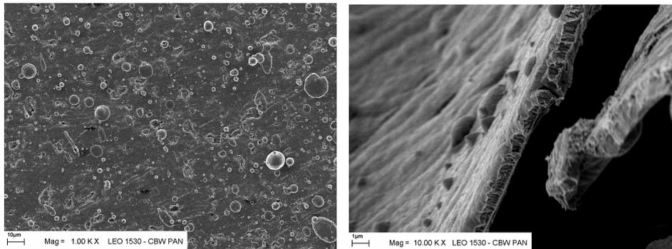
*Fig.10. SEM pictures showing a relatively large population of the deposited micro-droplets (left), and the edge and thickness of the deposited Nb-layer (right, larger magnification).*
