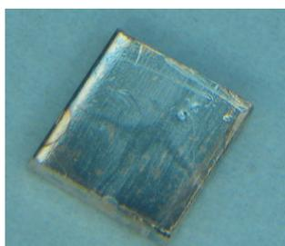
*Fig.24. Surface of the prepared Cu-sample after its Nb-coating and HPWR at 80 bars*
