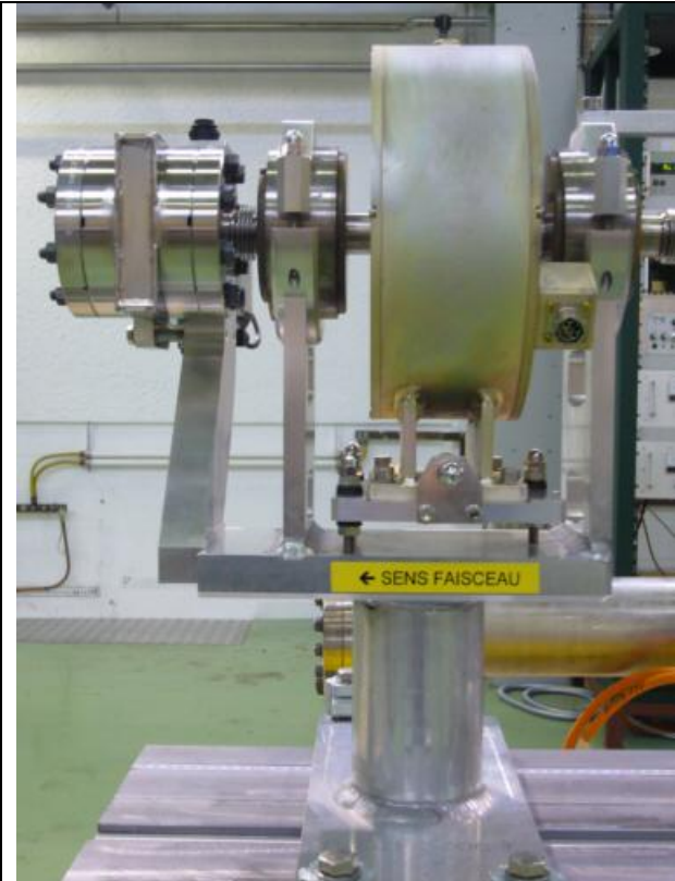
Sector 10: Beam Current Transformer between two quadrupoles, with sector valve at the beam exit.
