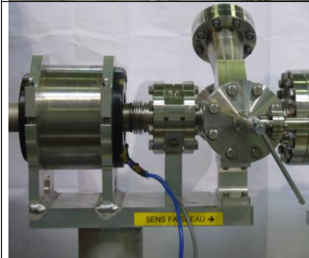
Sector 6: Beam pick-up and wire scanner.
