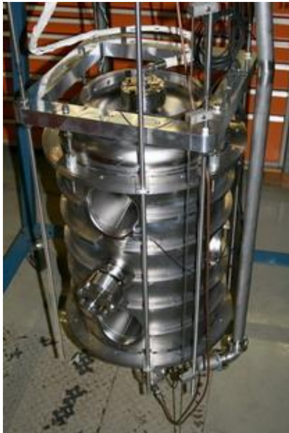
Figure 18 : Triple-spoke cavity at FZJ test stand.
