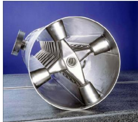
Figure 29 : Photo of the CH prototype before welding of the end cells
