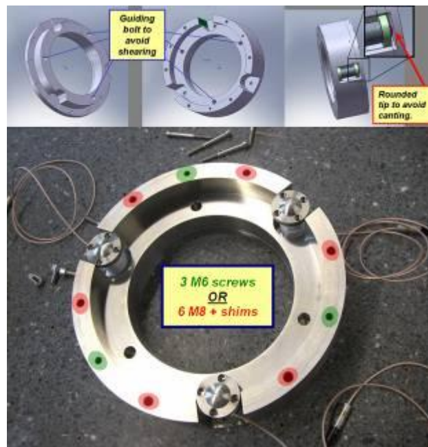
Figure 33 : Scheme of the piezo tuner on top and one part of the tuner carrying the three piezo actuators
