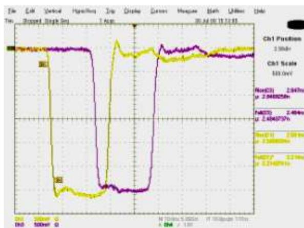
Figure 21: Chopper input and output waveforms
