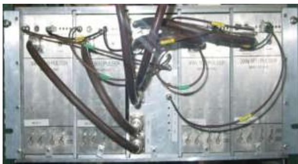
Figure 13: CERN driver  $\pm 250$  V prototype.
