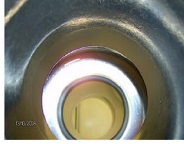
Fig. 6. Nb coated inner surface of the fourth, 1.3 GHz copper cavity, awaiting measuring in Jlab.
