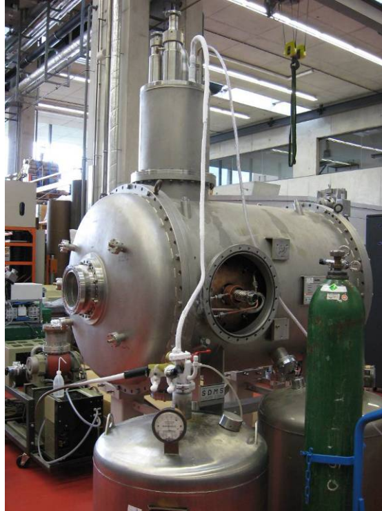
Figure 15: Cold test of the horizontal cryostat with liquid nitrogen.
