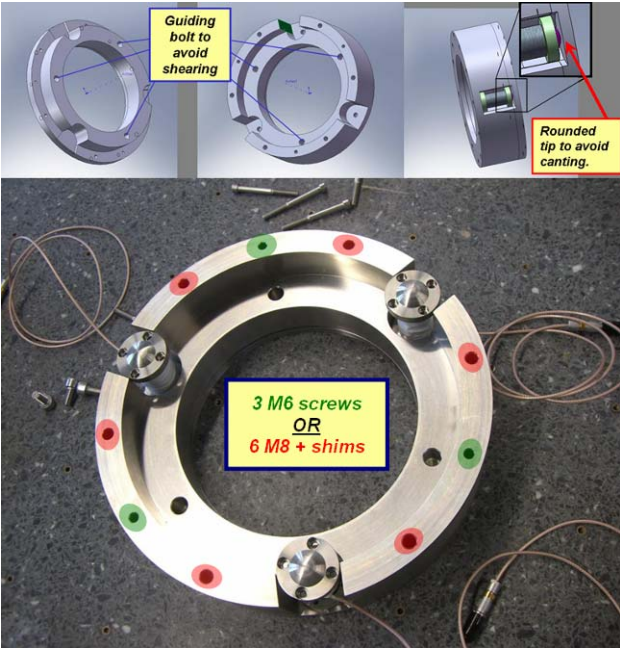
Figure 5: Scheme of the piezo tuner on top and one part of the tuner carrying the three piezo actuators below.
