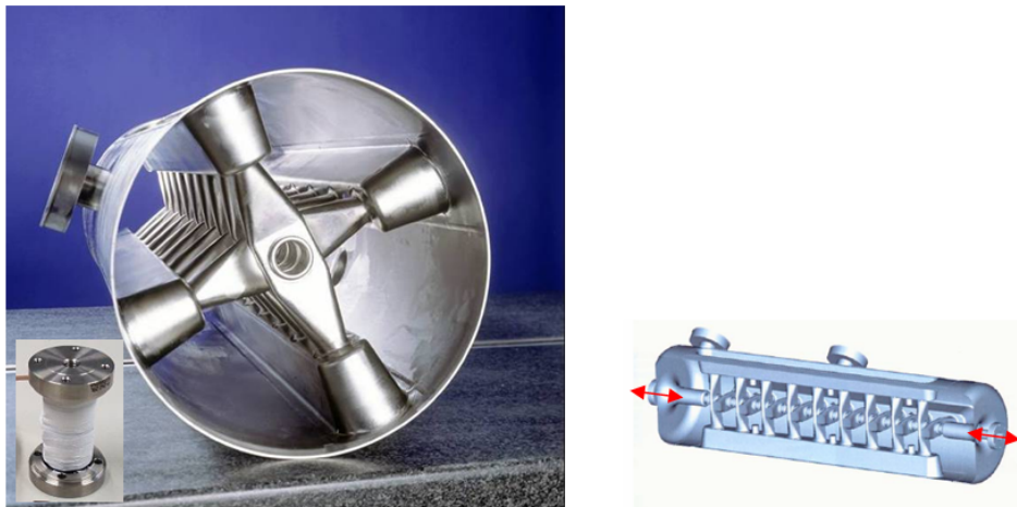
Figure 1: CH-prototype and investigated piezo actuator for application of tuning forces (red arrows).
