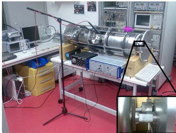
Figure 8: Setup for microphonics measurements at room temperature. The actuating piezo is installed between an endplate of the outer corset and the cavity near the beam pipe.
