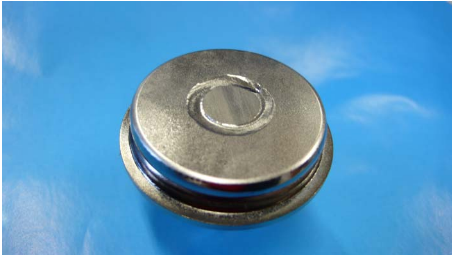
Figure 20: Membrane tuner, prototype for mechanical tests.
