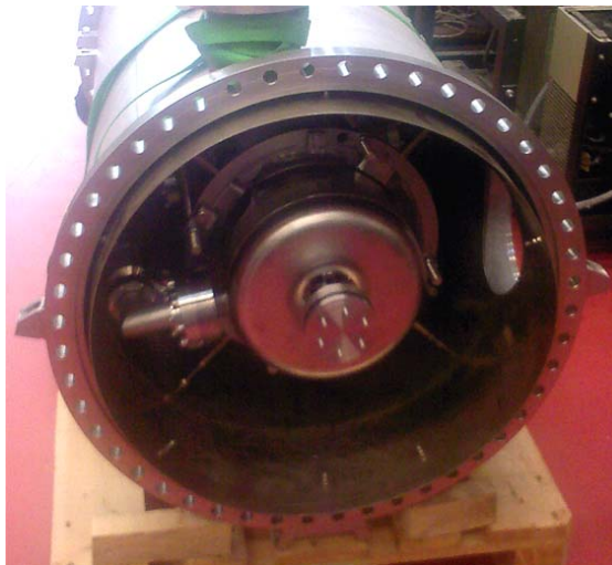
Figure 16: CH-prototype within the inner cold mass including \mu -metal shielding.
