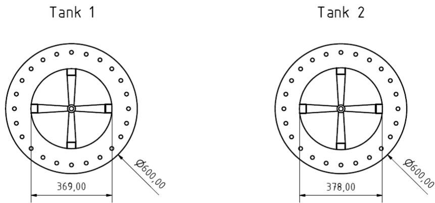
Fig. 4: Cross sectional view of the two acceleration structures of coupled cavity no. 2
