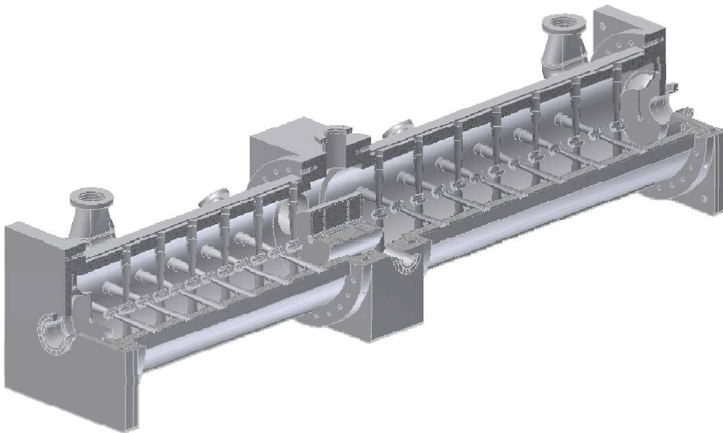
Fig. 1: 3d view into the coupled cavity no. 2 to be built as a prototype cavity
