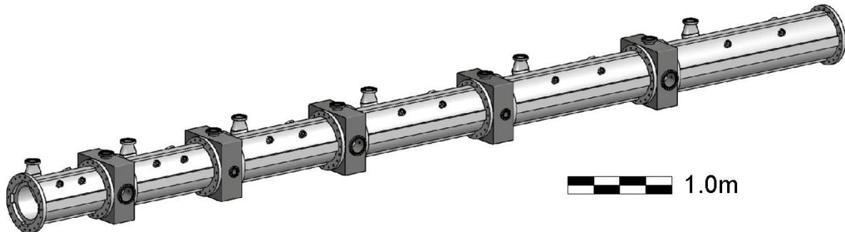
Fig. 2: View on the 35 MeV low power section of the proton linac, consisting of coupled CH-cavities no. 1, 2, 3.
