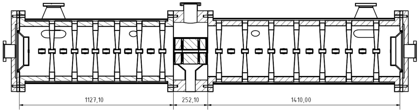
Fig. 3 Cross sectional view of coupled cavity no. 2
