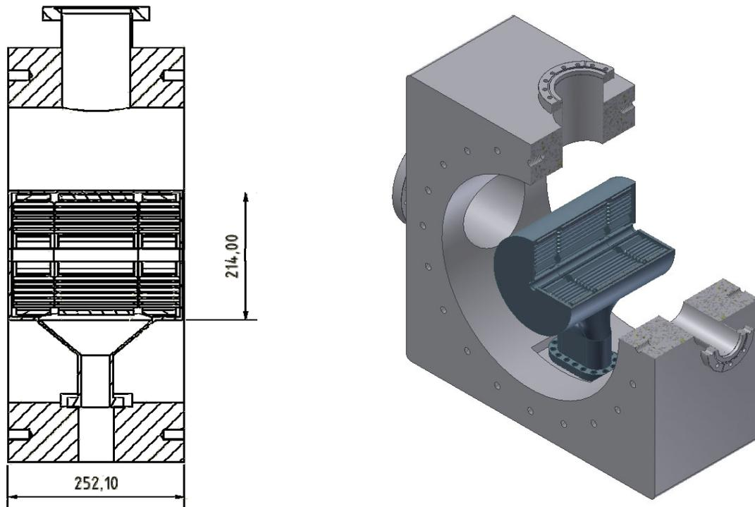
Fig. 7: Views of the coupling cell with internal quadrupole triplet
