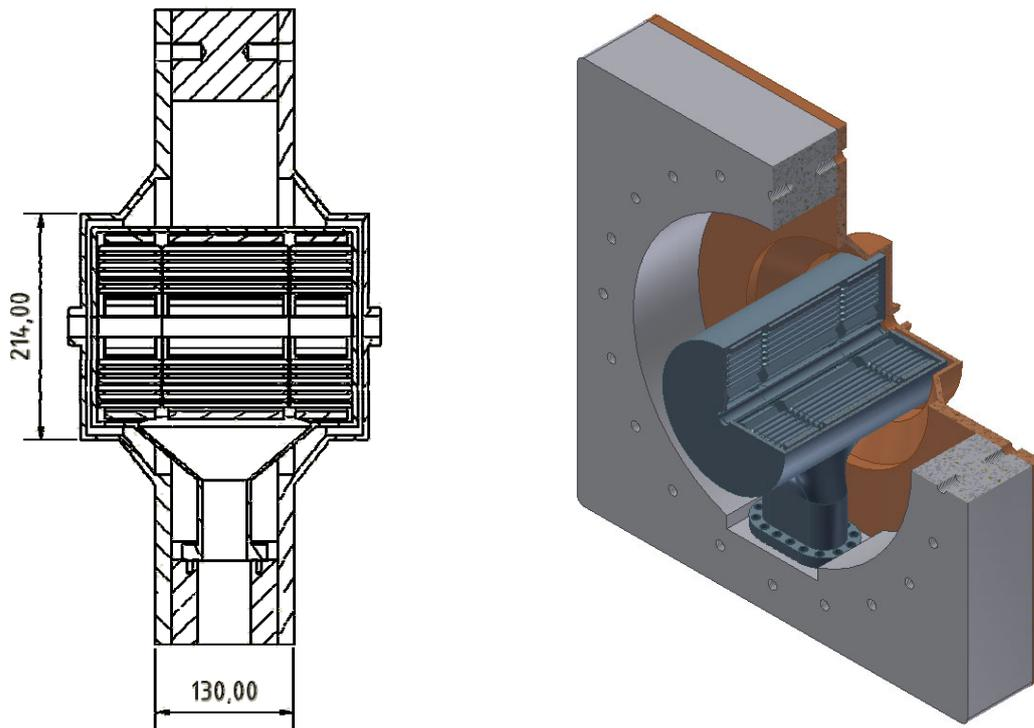
Fig. 6: Intertank unit between coupled cavities 1, 2, 3 in section no. 1)
