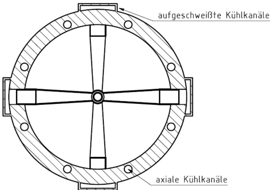
Fig. 10: Cooling channels in a cross sectional view
