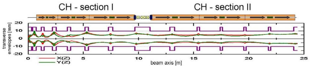
Fig. 5: 99% beam envelopes at 45mA of the whole 70 MeV DTL
