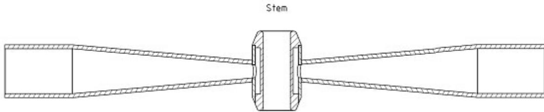
Fig. 8: Cross sectional view of a watercooled stem with drift tube
