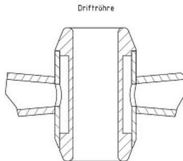
Fig. 9: - Detail of a water cooled drift tube
