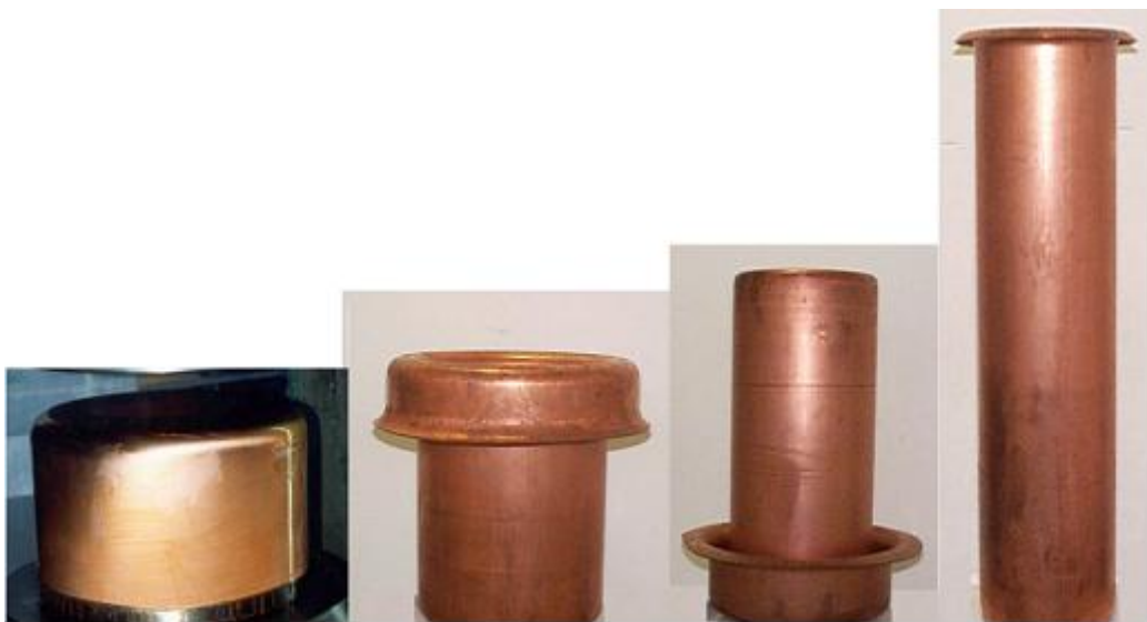
Figure 5: Reverse deep-drawing of seamless tubes. During each redrawing, the external surface of the cup to be drawn becomes the internal of the drawn part.
