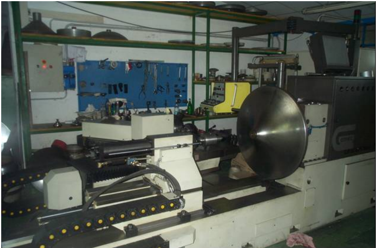
Figure 7: The spinning lathe used for the fabrication of seamless cavity prototypes. The lathe has only one turret which holds the rollers.
