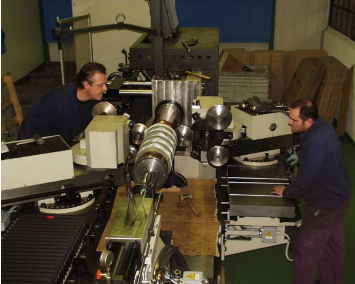
Fig. 9: Phase of the double turret necking process during the spinning parameter definition action.
