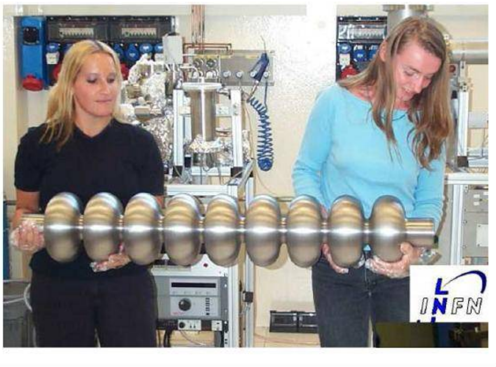
Figure 14 Niobium 9-cell cavity fabricated by spinning technology
