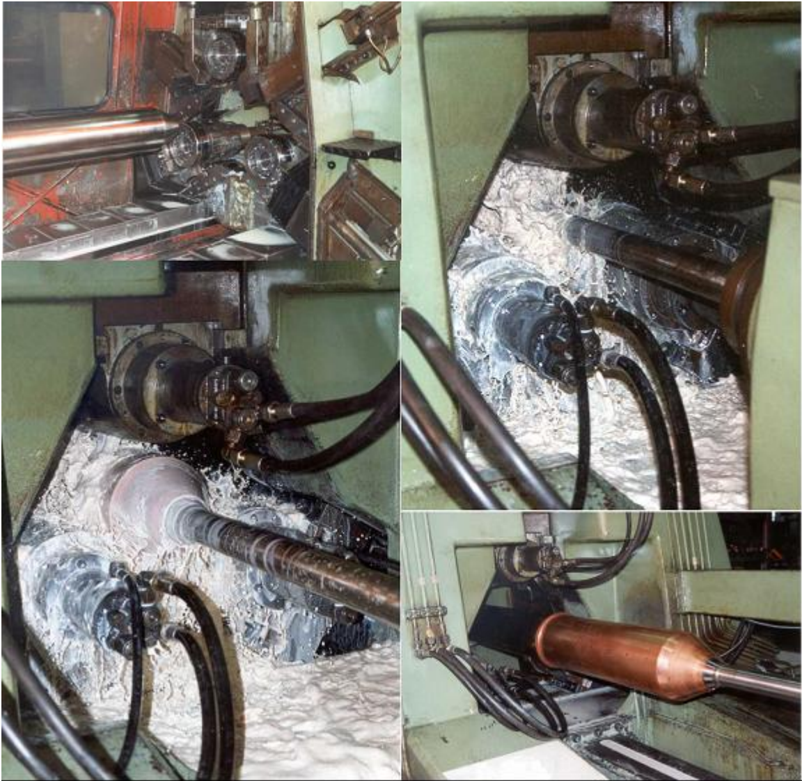
Figure 6: Forward flow-turning of seamless tubes. A short, thick tube is spun or drawn from a planar disc
