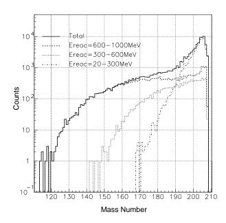
Fig. 3 Residue mass spectrum for p-induced reactions in a thick cylindrical <sup>*nat*</sup>Pb target (L = 100 cm, R = 10 cm) at 1 GeV incident energy. The calculation is performed with the Bertini code. Full line: total spectrum, dashed, dotted and dashed-dotted lines: reactions induced by particles of kinetic energy in the bin 600-1000 MeV, 300-600 MeV and 20-300 MeV, respectively.
