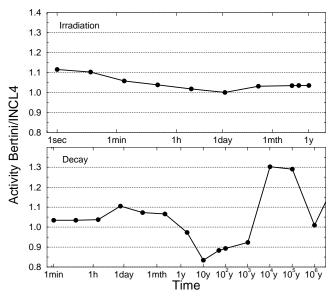
Fig. 6 Ratio of the activities given by the Bertini and INCL4 calculations, during the irradiation (top) and decay (bottom) phases.
