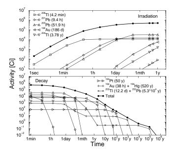
**Fig. 4** Total and partial activities of a <sup>*n* a *t*</sup> Pb target as a fonction of irradiation time (top) and cooling time (bottom) with the Bertini cascade model.
