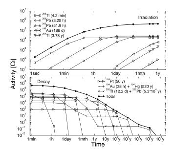
Fig. 5 Same as Fig. 4 for a calculation with the INCL4 cascade model.
