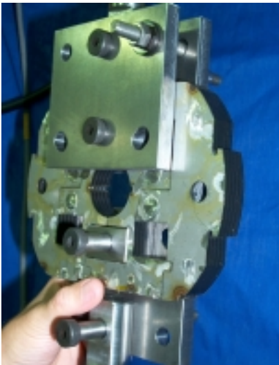
Fig. 4. A sample for tensile test during fixture assembly. This sample consists of alternated lamination assembled, welded and impregnated.
