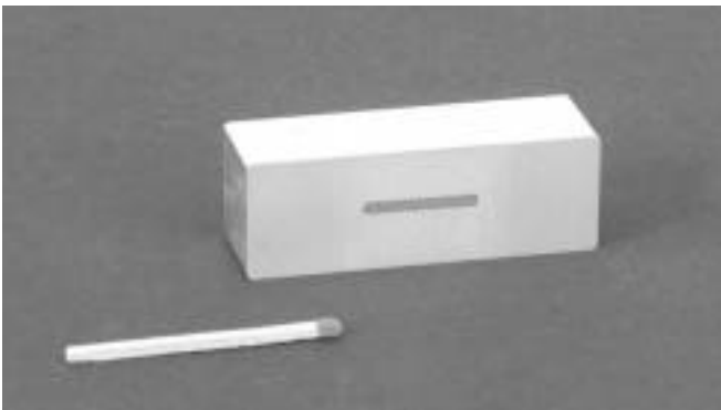
Fig. 4. The CMS conductor after electron beam welding and machining. The conductor dimensions are 21.6 mm \times 64.0 mm.
