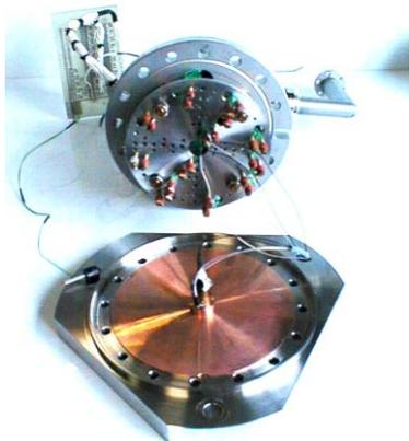
Figure 2 : The thermometric system including the thermometers array and the calibration heater mounted of the backside of a Nb/Cu sample.
