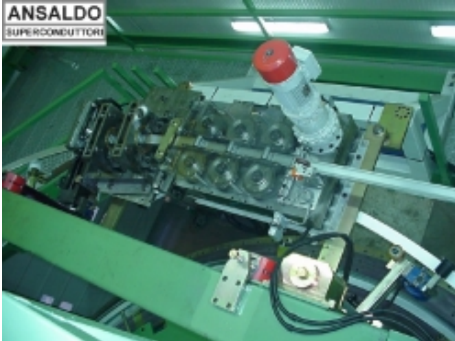
Fig. 5. The constructed two-step pre-bending unit under test.
