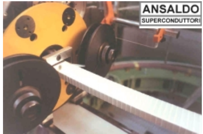
Fig. 7. Taping unit mounted in the winding line.
