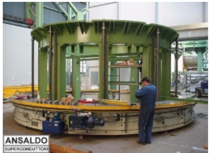
Fig. 8. Winding table with fixed and rotating parts and lifting system.
