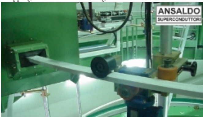
Fig. 6. Conductor coming out from sandblasting unit during operation.
