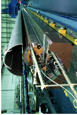
Shell-welding preparation for 14-m-long, twin-aperture LHC arc dipole magnet at CERN
