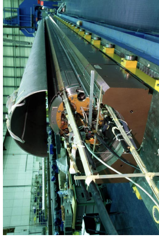
Shell-welding preparation for twin-aperture, 15-m-long LHC arc dipole magnet at CERN
