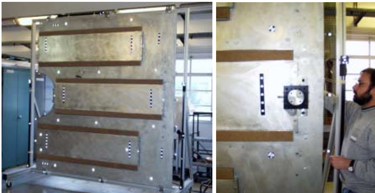
Figure 4 : Left : Aluminum mock up of the central part of Station 5 (at scale 1). The different types of surveyor's target are shown. Right : Tuning of the slat positioning system on the panel support.
