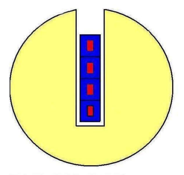
R(Ga) = 128 cm; W-shielding: D 32 x (4 x 35) cm; Overall dimensions of Zr tube/cooling system: D 47 x 175cm
