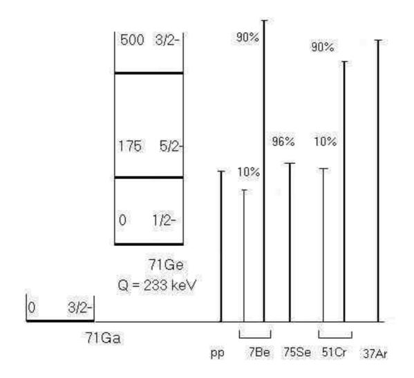
Fig.1. Level scheme for 71Ge showing the excited states that contribute to absorption of pp. 7Be, 75Se, 51Cr and 37Ar neutrinos.
