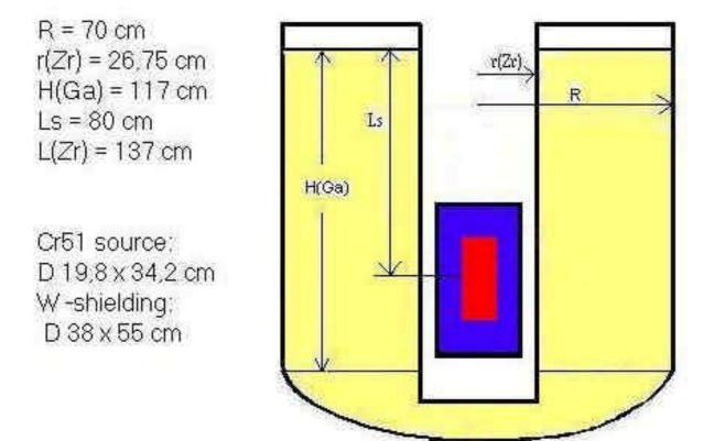
Fig.6. Geometry of new SAGE calibration experiment with single GALLEX source.
