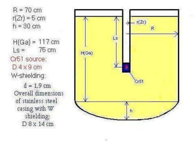
Fig.4. Geometry of SAGE calibration experiment.
