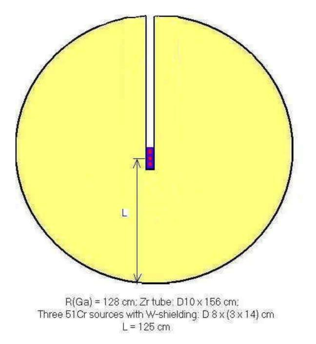
Fig.9. Geometry of the calibration source with 50 t of Ga and SAGE's composite source (3 compact sources).
