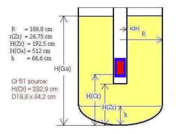
Fig.2. Geometry of GALLEX calibration experiment(s).
