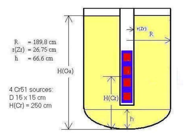
Fig.3. Geometry of new GALLEX calibration experiment.
