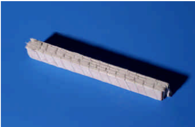
Stack of \text{Nb}_3\text{Sn} cables insulated with CEA/Saclay innovative pre-impregnated fiber tape after heat treatment (Courtesy L. Girard).
