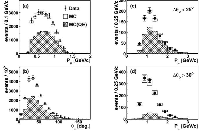
Figure 9: *muon momentum and angle distribution from CC neutrino cross sections in  $H_2O$  as measured by the K2K front detectors: KT thus to be constrained as precisely as possible. The shaded area represents the MC predicted QE fraction.*
