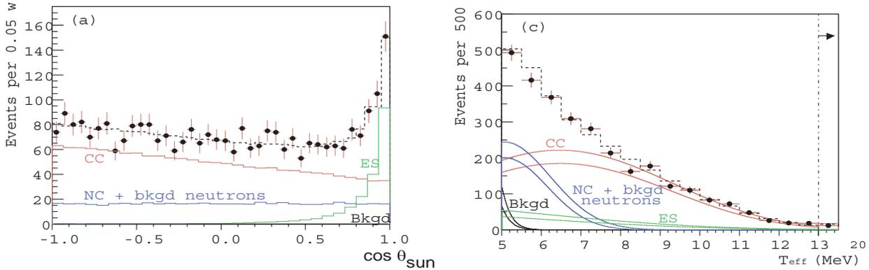
Figure 5: *Distribution of  $\cos \theta_{\text{sun}}$  and electron kinetic energy, compared with NC, ES, CC Monte Carlo predictions assuming SSM neutrino spectrum shape.*
