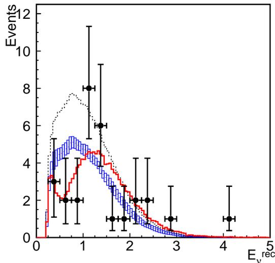
Figure 10: *Reconstructed neutrino energy for the 29 1-ring  $\mu$ -like events measured by K2K; compared with a no-oscillation spectrum, Blue Box histogram (resp. dashed curve) normalized to the observed (resp. expected) number of events and the best fit oscillation analysis (red curve).*
