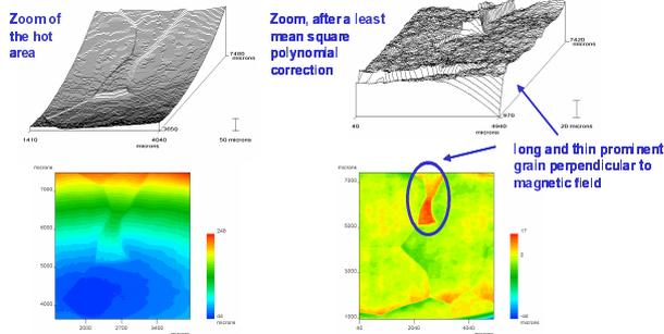
**Figure 5: example of a morphological defect found in the vicinity of the quench (localized by a temperature map)**
