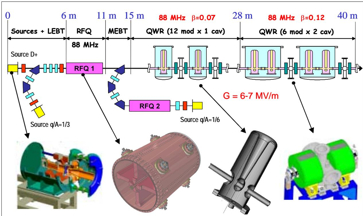
**Figure 1: Architecture of the SPIRAL 2 Linac**
