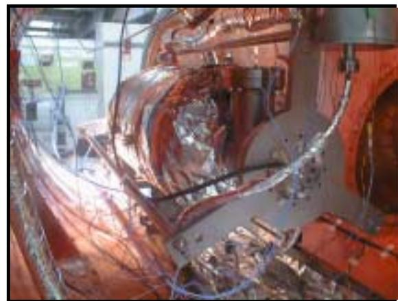
**Figure 3: Test in CryHoLab: 700 MHz 5-cell cavity for proton Linac**
