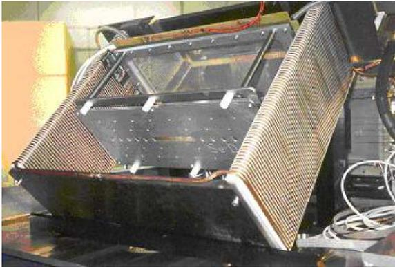
Fig. 1. The picture shows the detector Se-D mounted at the focal plane of Vamos. In the foreground, we see the mask, behind which is the emissive foil, the frame of the accelerating grid, the detector located 20 cm further. The unit is placed in a coil which induces a longitudinal magnetic field in the drift volume. The device is placed at  $45^\circ$  with respect to the incident ions.
